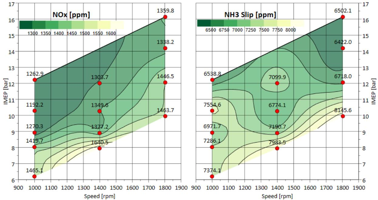
Figure 7 Emissions of NO<sub>x</sub> and ammonia slip for pure ammonia test region
