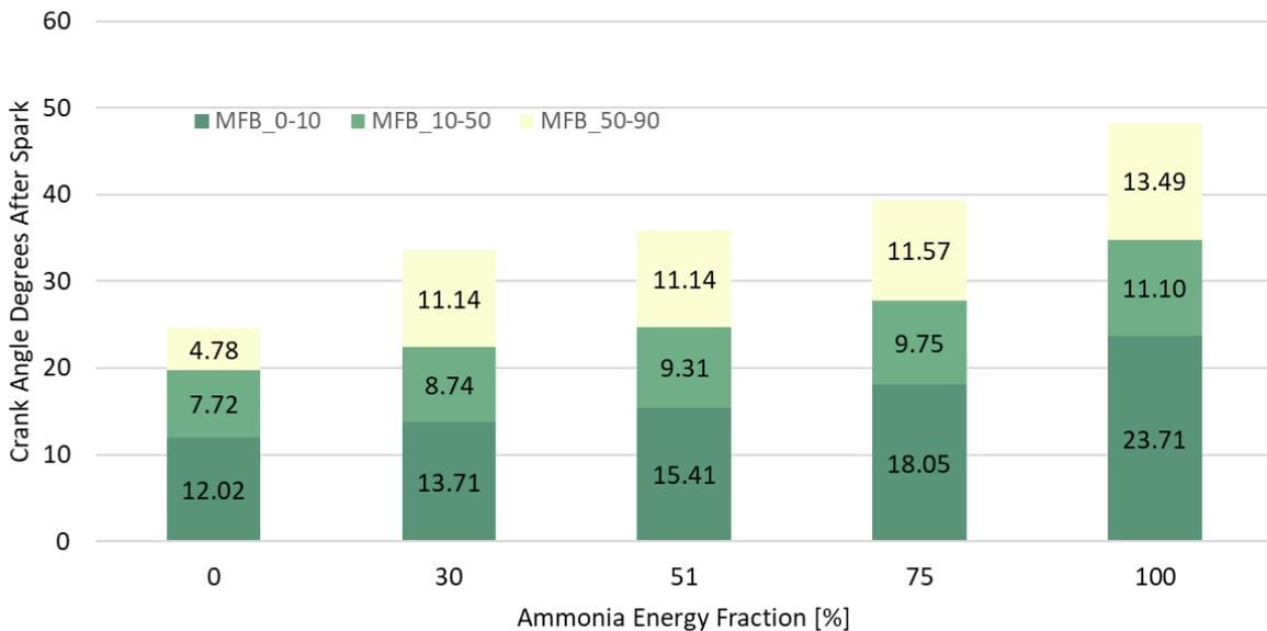
**Figure 9 Combustion metrics for different levels of ammonia substitution**
