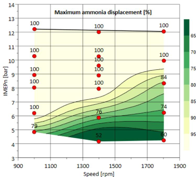
**Figure 3 Maximum substitution of ammonia achieved at different load points ( $\lambda=1$ , MBT spark timing)**
