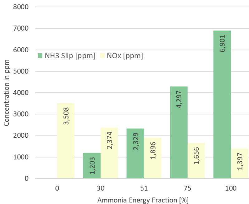
**Figure 11 Emissions of NO<sub>x</sub> and ammonia slip for various E10 substitution rates**
