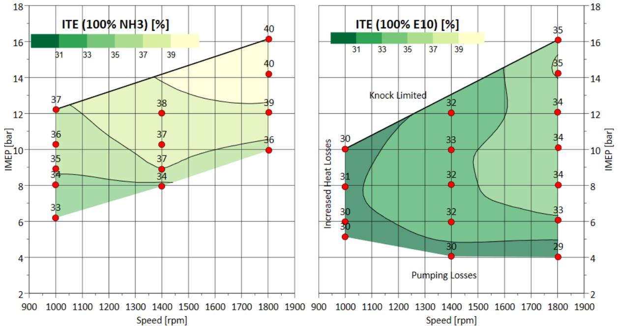
**Figure 6 ITE of 100%  $\text{NH}_3$  vs 100% E10 operation**
