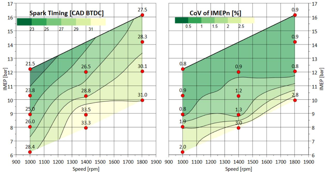
Figure 4 Spark timing and CoV of IMEPn of pure ammonia test points
