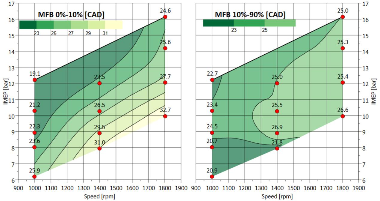
**Figure 5 Variation of combustion metrics 0%-10% MFB and 10%-90% MFB for pure ammonia combustion at various speeds and loads**
