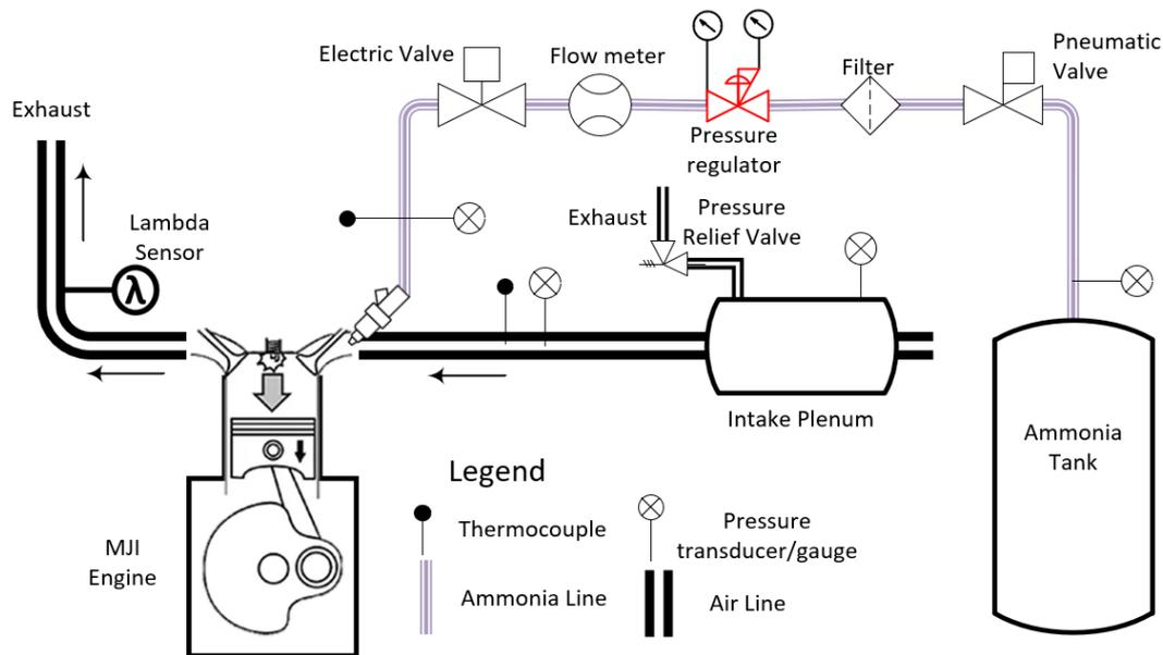
**Figure 2 Schematic of the engine fuel supply line**
