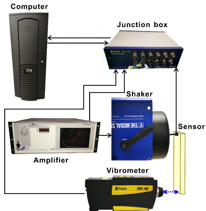
Fig. 2 Schematic diagram of the FRFs testing system
