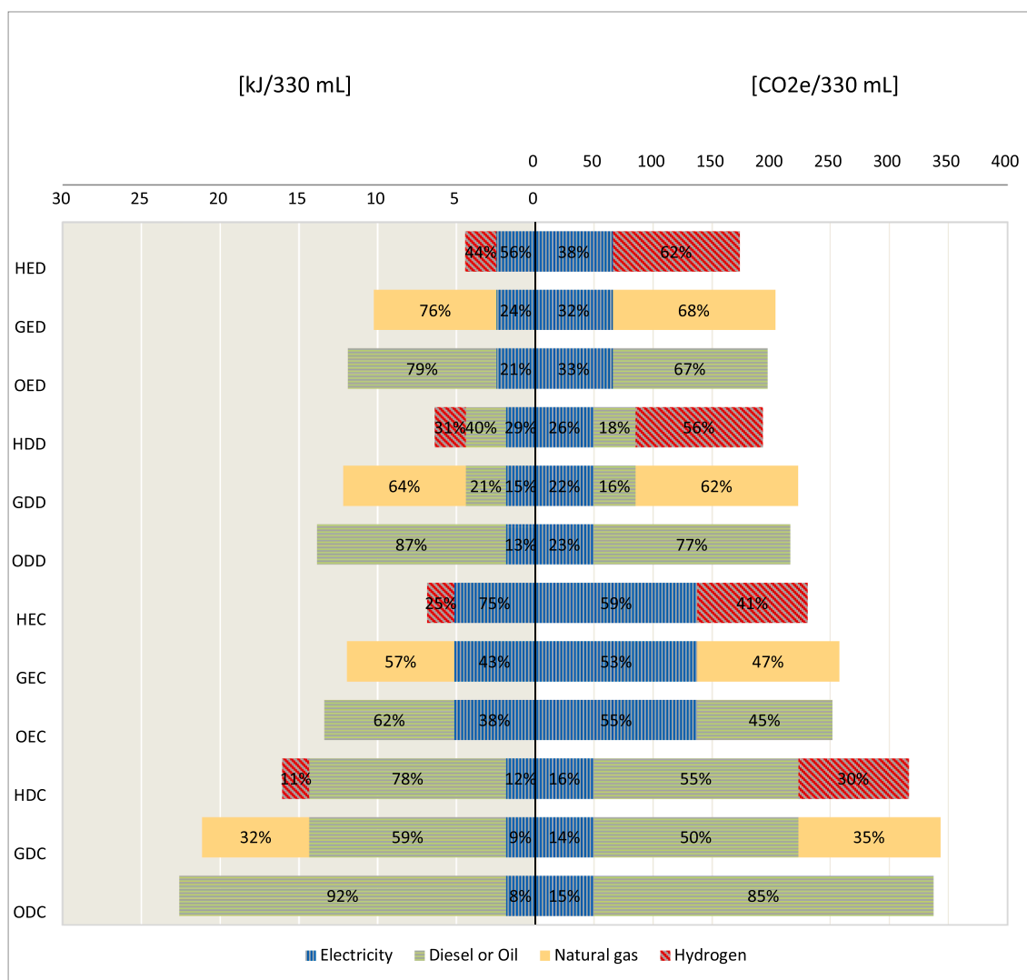
Fig. 11. Energy use [kJ] (right side) and emissions from energy use [CO 2 e] (left side) per 330 ml of cream manufacturing and distribution in 2020 under 12 scenarios of Table 6. The figure also presents the energy mix between the different energy resources used in each scenario.
