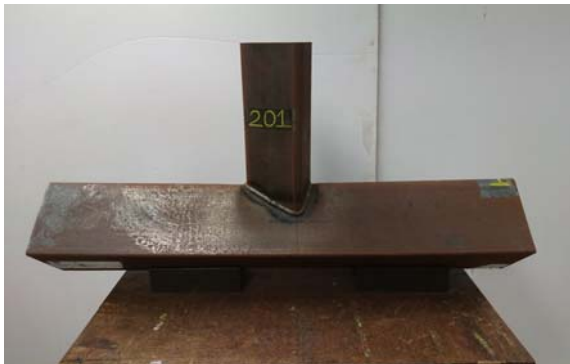
(a) Comparison of test and FE DBB T-joint ( \omega=27^\circ ) failed by chord crown failure (C) mode.
