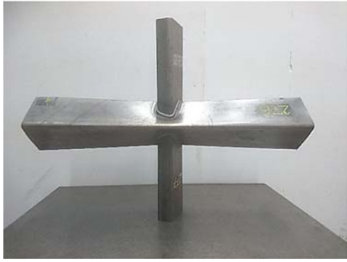
(c) Comparison of test and FE DBB X-joint ( \omega=63^\circ ) failed by chord crown failure (C) mode. Figure 10. Failure mode comparisons between test and FE specimens of DBB X-joints.
