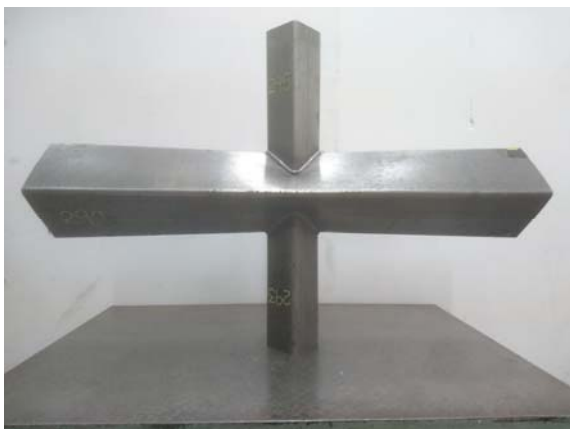
(b) Comparison of test and FE DBB X-joint ( \omega=45^\circ ) failed by chord crown failure (C) mode.
