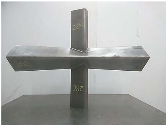
(a) Comparison of test and FE DBB X-joint ( \omega=27^\circ ) failed by chord crown failure (C) mode.
