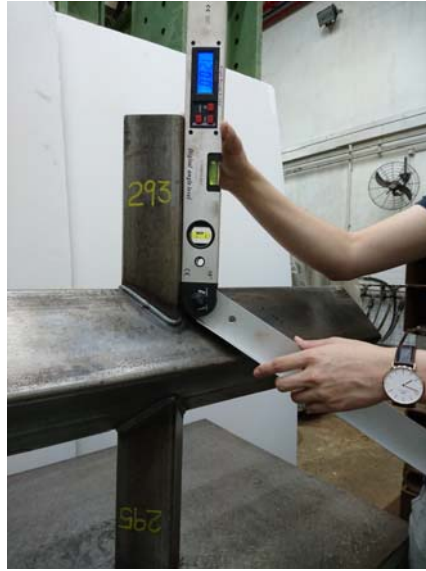
Figure 2. Dihedral angle ( \psi=120^\circ ) for DBB X-joint (also valid for DBB T-joint).
