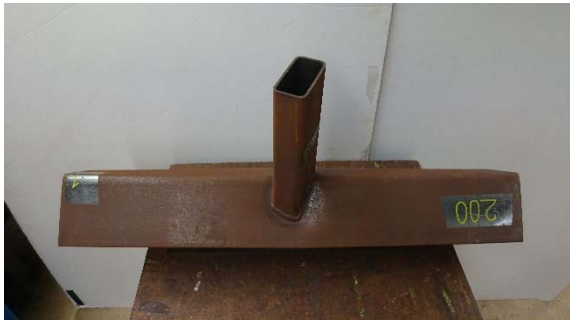
(c) Comparison of test and FE DBB T-joint ( \omega=63^\circ ) failed by chord crown failure (C) mode. Figure 9. Failure mode comparisons between test and FE specimens of DBB T-joints.
