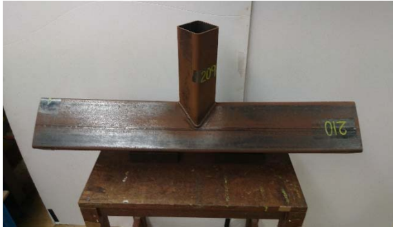
(b) Comparison of test and FE DBB T-joint ( \omega=45^\circ ) failed by chord crown failure (C) mode.
