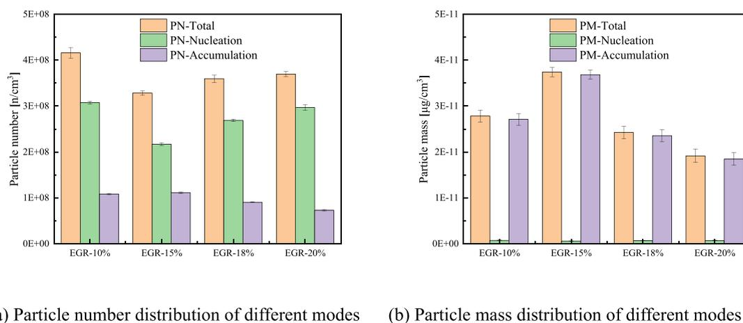
**Figure 8.** Characteristic of particle emission distribution at various EGR rates for 0.2 IOC.
