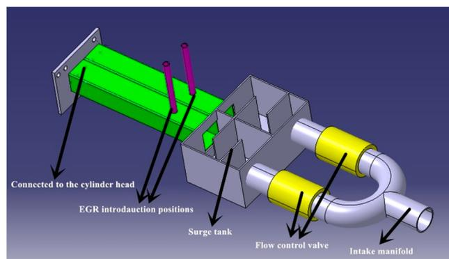
Figure 14. Intake stratification device.
