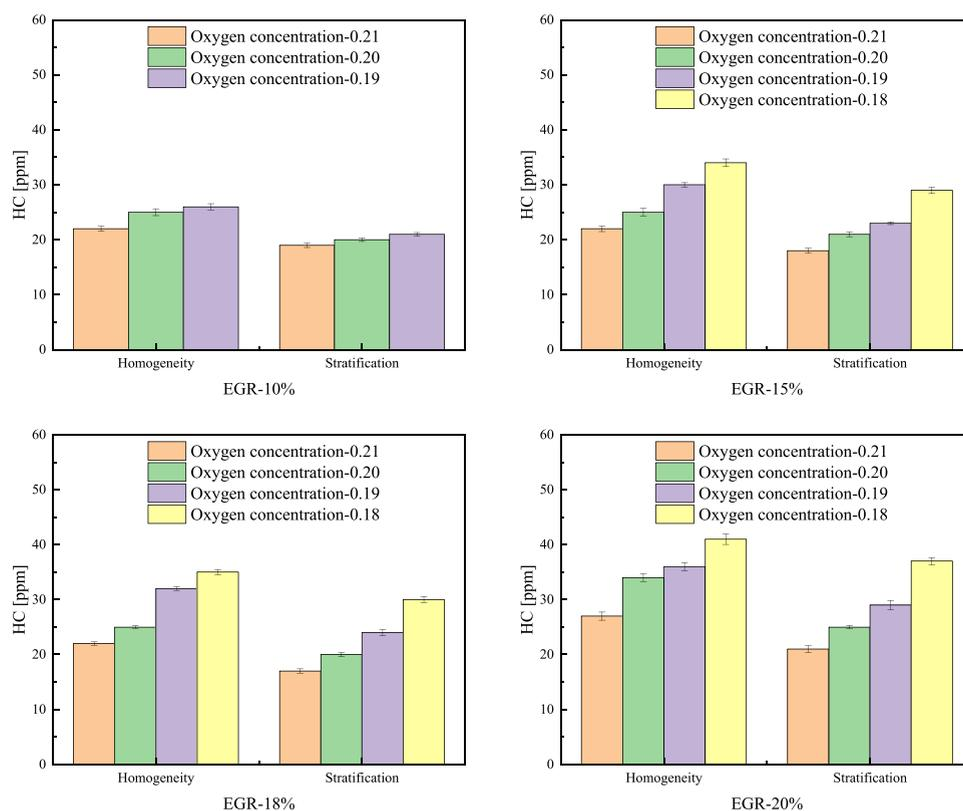
**Figure 13.** HC emissions with different intake forms and components.
