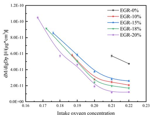
Figure 4. PM emissions with various intake components.
