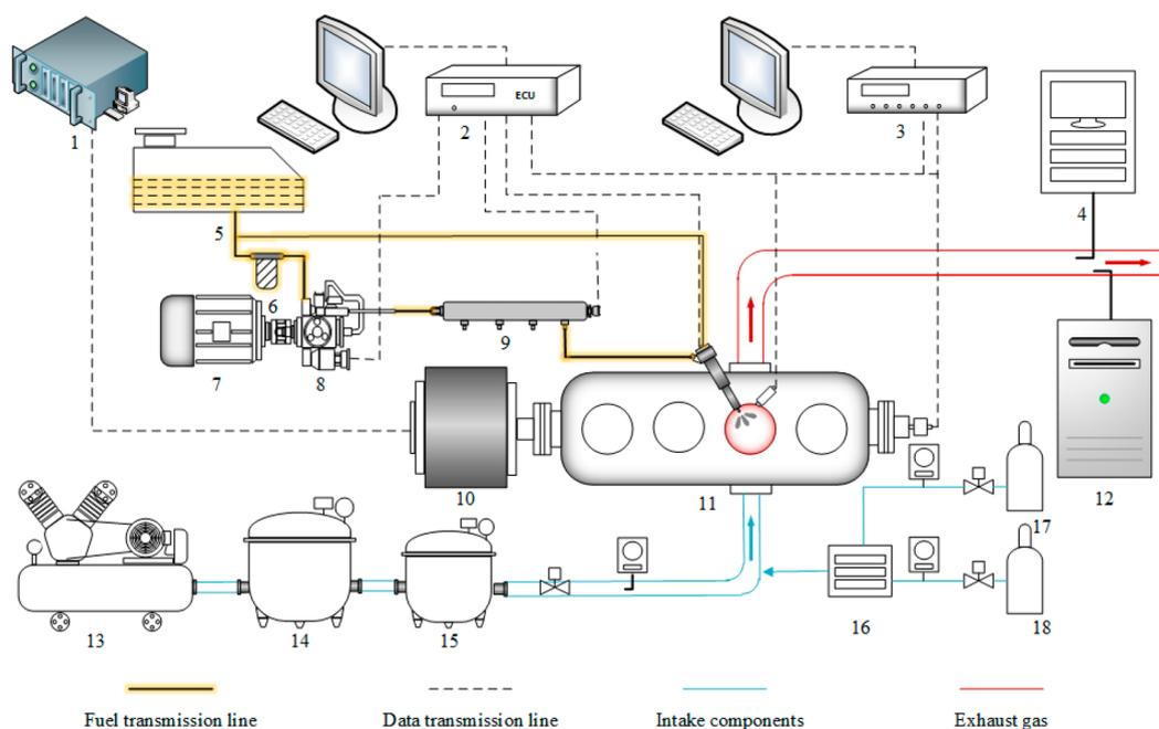
1: dynamo controller; 2: ECU (NI2106); 3: combustion analyzer; 4: CMBUSTION fast exhaust gas analyzer; 5: fuel tank; 6: filter; 7: fuel pump motor; 8: high pressure fuel pump; 9: high pressure common rail; 10: dynamo meter; 11: test engine; 12: DMS500 particle size spectrometer; 13: air compressor; 14: primary regulator tank; 15: secondary regulator tank; 16: intake components control equipment; 17: high pressure O<sub>2</sub> cylinder; 18: high pressure CO<sub>2</sub> cylinder;
