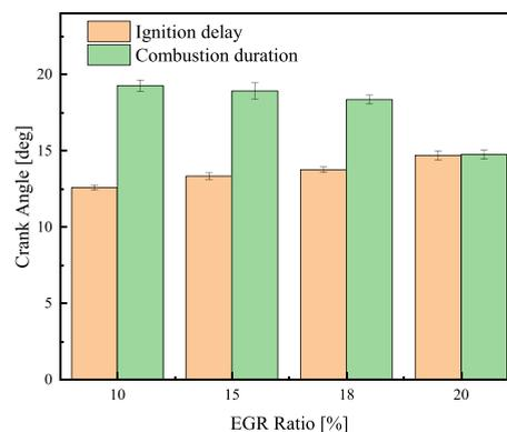
Figure 5. Ignition delay and combustion duration at various EGR rates for an IOC value of 0.2.
