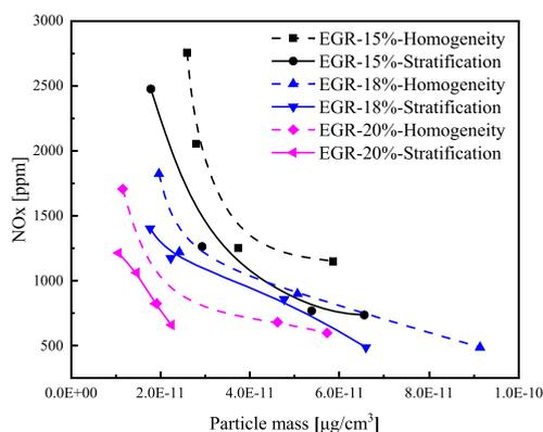
**Figure 12.**  $\text{NO}_x$  and PM emissions with different intake configurations and components.
