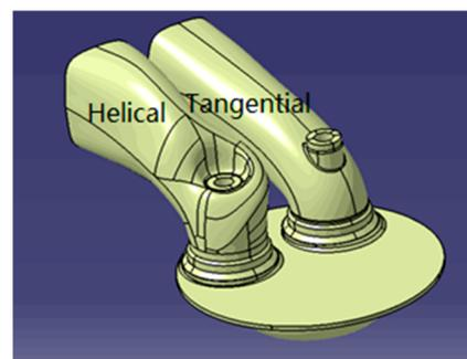
Figure 15. Three-dimensional model of the intake port.
