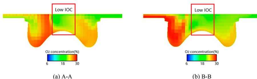
**Figure 11.** Distribution of oxygen concentration in the cylinder at 8 °CA BTDC: (a) A–A direction and (b) B–B direction.
