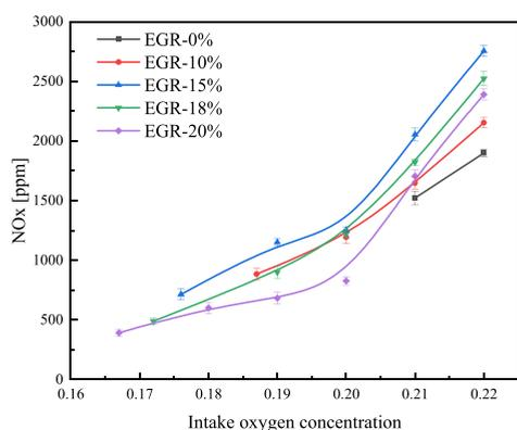
Figure 3. NO<sub>x</sub> emissions with various intake components.
