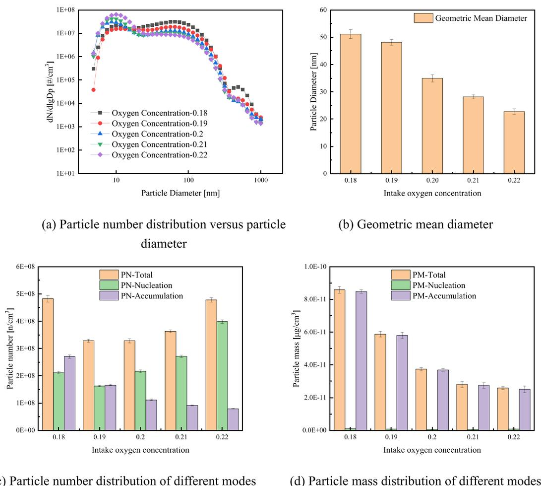
**Figure 7.** Characteristics of particle emission distribution at various IOCs for a 15% EGR rate.
