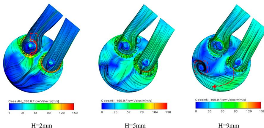
**Figure 10.** Distribution of the velocity field in the cylinder at different times during the intake process.
