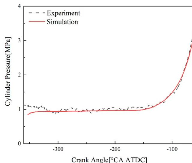
**Figure 9.** Comparison of in-cylinder pressure curves between simulation and experiment.
