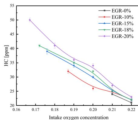
Figure 6. HC emissions with various intake components.
