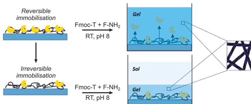
**Figure 9.** Reversible and irreversible enzyme immobilization on modified surfaces for biocatalytic self-assembly. Irreversible enzyme immobilization confines gel formation to the vicinity of the surface while reversible enzyme immobilization leads to gelation of the bulk material. Reproduced with permission from ref 91. Copyright 2017, American Chemical Society.
