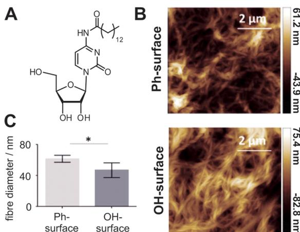
**Figure 6.** Films of fibers formed from a cytidine-based gel film on hydrophilic glass (OH) and hydrophobic phenyl (Ph) surfaces. (A) Structure of the gelator. (B) AFM images of the fibers formed on OH and Ph surfaces. (C) Average diameter of the fibers on the OH and Ph surfaces as measured by AFM. Reproduced with permission from ref 74. Copyright 2016, Royal Society of Chemistry.
