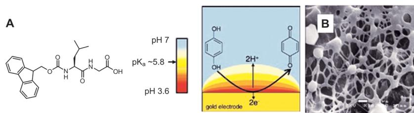
**Figure 7.** Electrochemically grown Fmoc-LG gel film. (A) Molecular structure of Fmoc-LG and electrochemical oxidation of hydroquinone to trigger near-surface gelation. (B) Cryo-SEM image of the top surface of the gel film. Reproduced with permission from ref 80. Copyright 2010, American Chemical Society.
