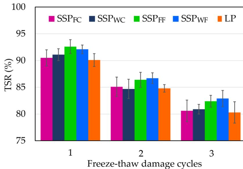
**Fig. 11** TSR results of asphalt mixtures
