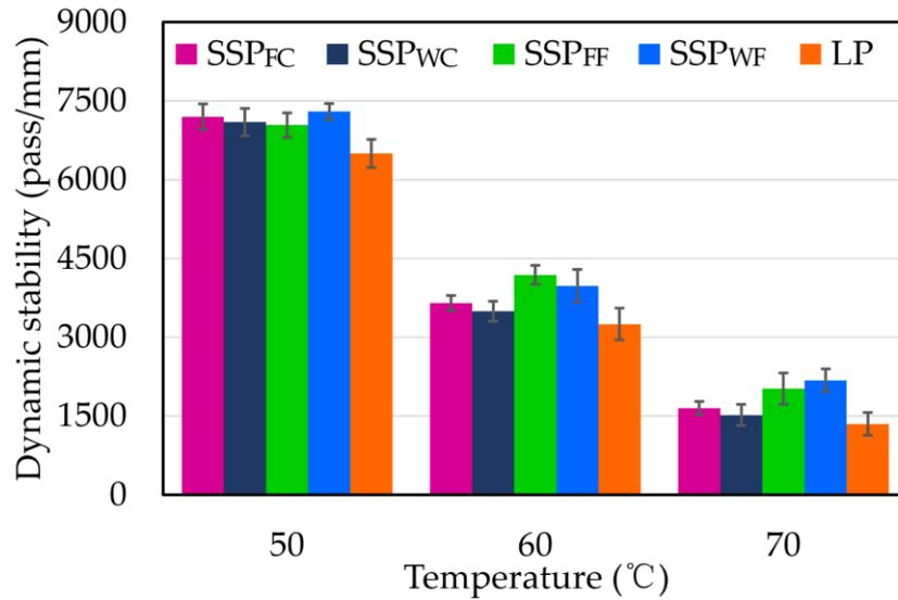
**Fig. 12** Dynamic stability results of asphalt mixtures
