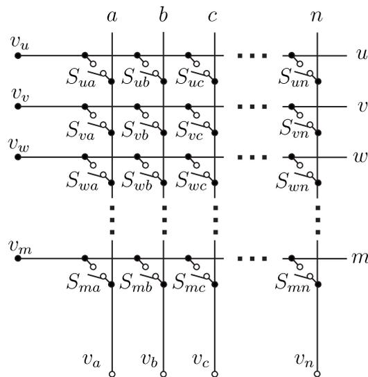
Figure 17. An  $m \times n$  direct matrix converter.
