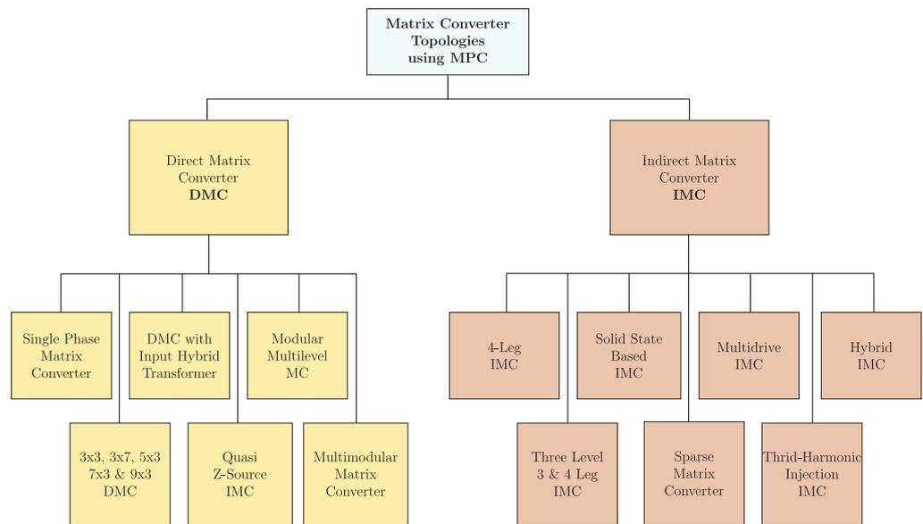
Figure 15. Classification of matrix converters.
