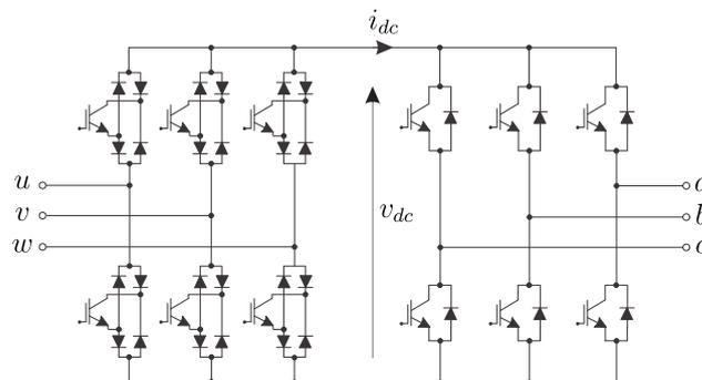
Figure 25. Sparse matrix converter.
