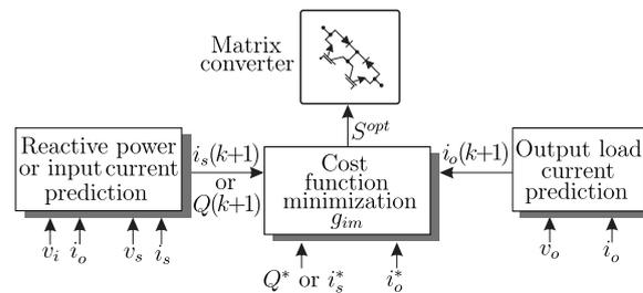
Figure 8. Predictive current control with input resonances mitigation block diagram.
