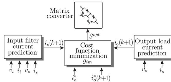
Figure 7. Predictive current control with imposed input current block diagram.
