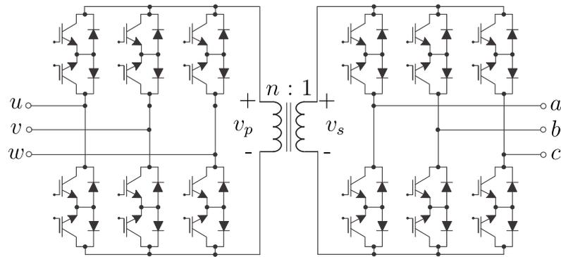
Figure 26. Solid-state-transformer-based matrix converter.
