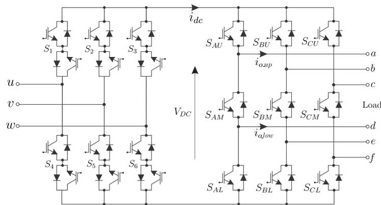
Figure 28. Indirect matrix converter with dual output.
