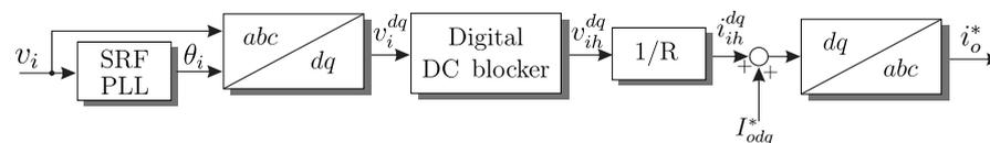
Figure 9. Output current reference generation for active damping approach.
