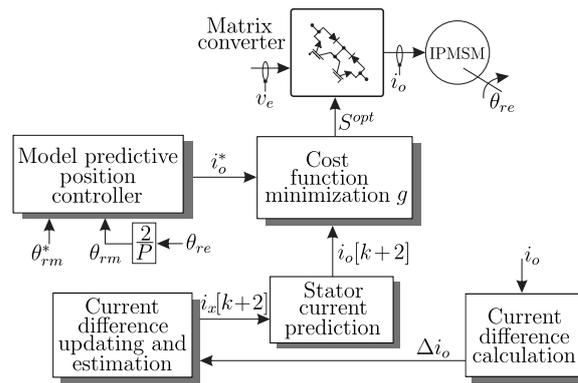
Figure 14. Predictive position and speed control block diagram.
