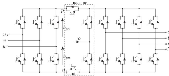
Figure 23. Three-level indirect matrix converter.
