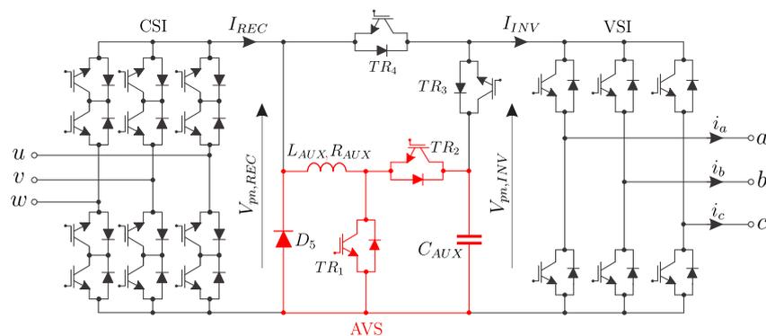
Figure 27. Hybrid indirect matrix converter.
