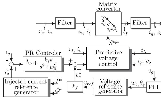
Figure 12. Predictive voltage control block diagram.
