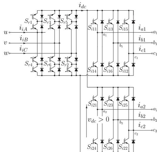
Figure 29. Multi-drive indirect matrix converter.
