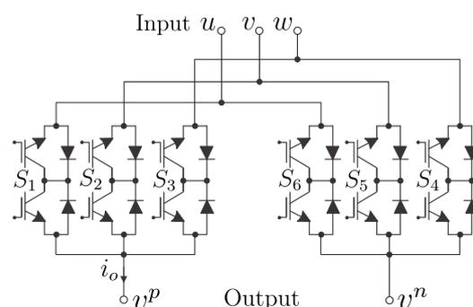
**Figure 16.** A single-phase matrix converter.
