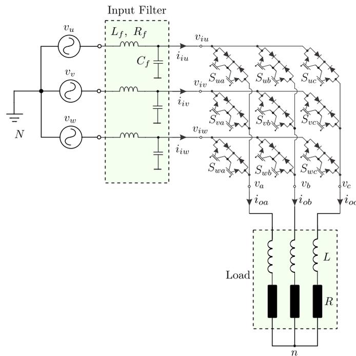
Figure 5. Three-phase direct matrix converter feeding an RL load.
