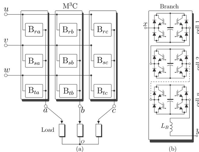
Figure 20. Modular multilevel matrix converter. (a) Generic M<sup>3</sup>C, (b) Branch composed by one inductor  $L_B$  and  $n$  full-bridges.
