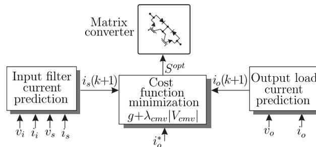
Figure 10. Predictive current control with common-mode voltage block diagram.
