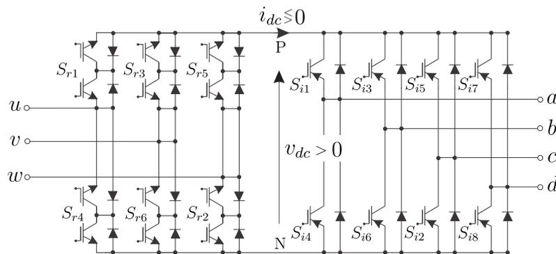
Figure 22. Four-Leg indirect matrix converter.
