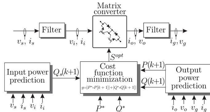
Figure 13. Predictive power control block diagram.
