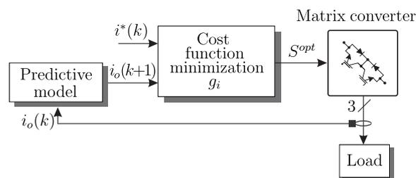
**Figure 4.** Predictive current control block diagram.
