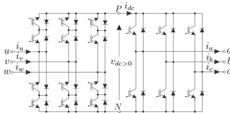
Figure 21. Power stage of an indirect matrix converter.
