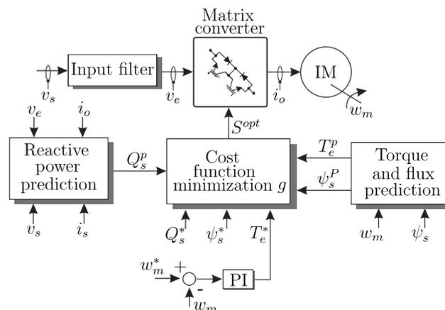
Figure 11. Predictive torque and flux control block diagram.
