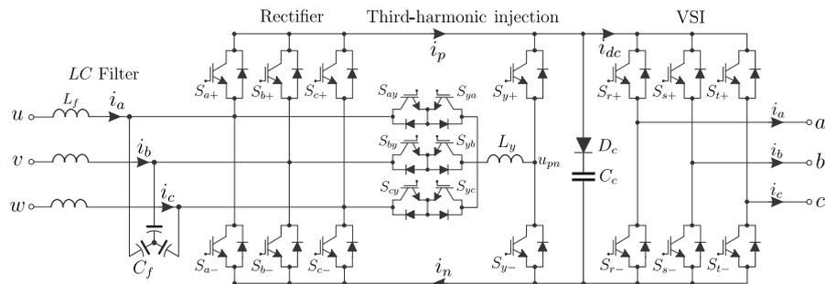
Figure 24. Two-stage matrix converter with third-harmonic injection.
