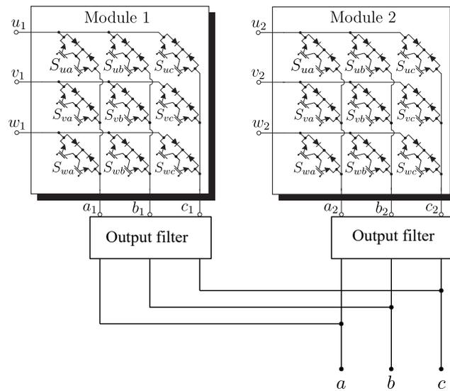
Figure 19. Multi-modular matrix converter.
