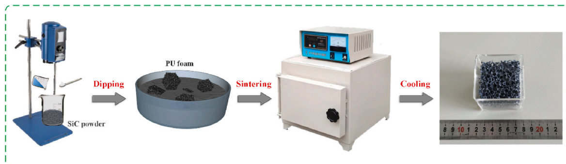
Fig. 1. Schematic of the preparation process of the ceramic foam.
