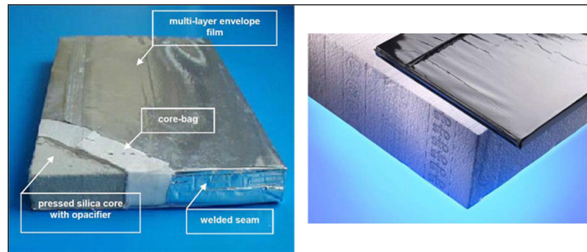
Figure 3. Visual presentation of a vacuum insulation panel (left) and a comparative material thickness with a traditional insulation (extruded polystyrene) achieving the same thermal conductivity level (right) [21,22].
