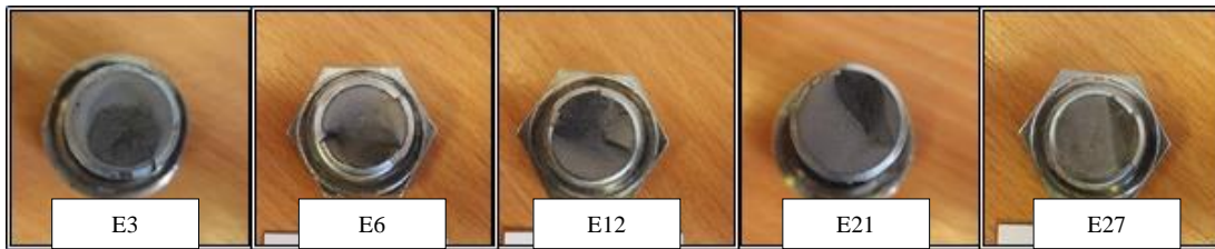
(a) \Delta\sigma_n / f_{yb} = 0.9 (b) \Delta\sigma_n / f_{yb} = 0.7 (c) \Delta\sigma_n / f_{yb} = 0.6 (d) \Delta\sigma_n / f_{yb} = 0.5 (e) \Delta\sigma_n / f_{yb} = 0.45
