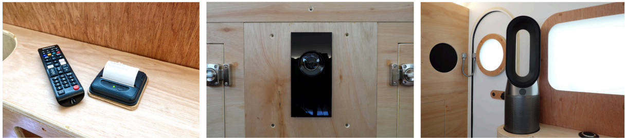
Figure 7. (Left image) The receipt printer provides a printed record of each experience, (middle image) a physical representation of the AI which guides the audience through the experience, (Right image) the smart fan which is used to collect air quality data and performs as part of the immersive experience.
