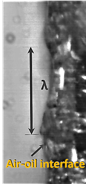
Fig. 10: Schematic diagram of the determination of the wave-length from the images.
