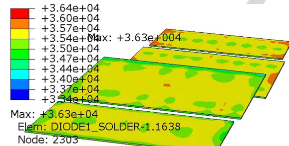
Step: T25, Cool down to 25C Increment 24; Step Time = 180.0 Primary Var: S, Mises
