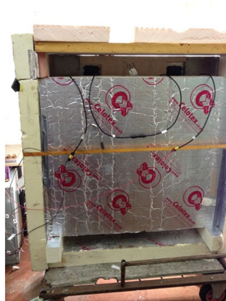
Figure 6. Photograph of insulation position and inlet and outlet of air duct.
