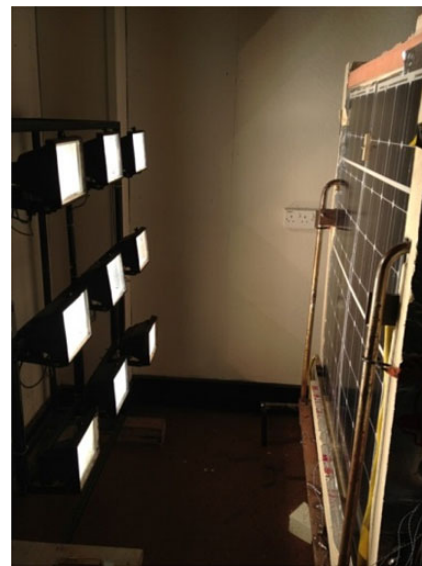
Figure 7. Photograph of artificial lights and their position.
