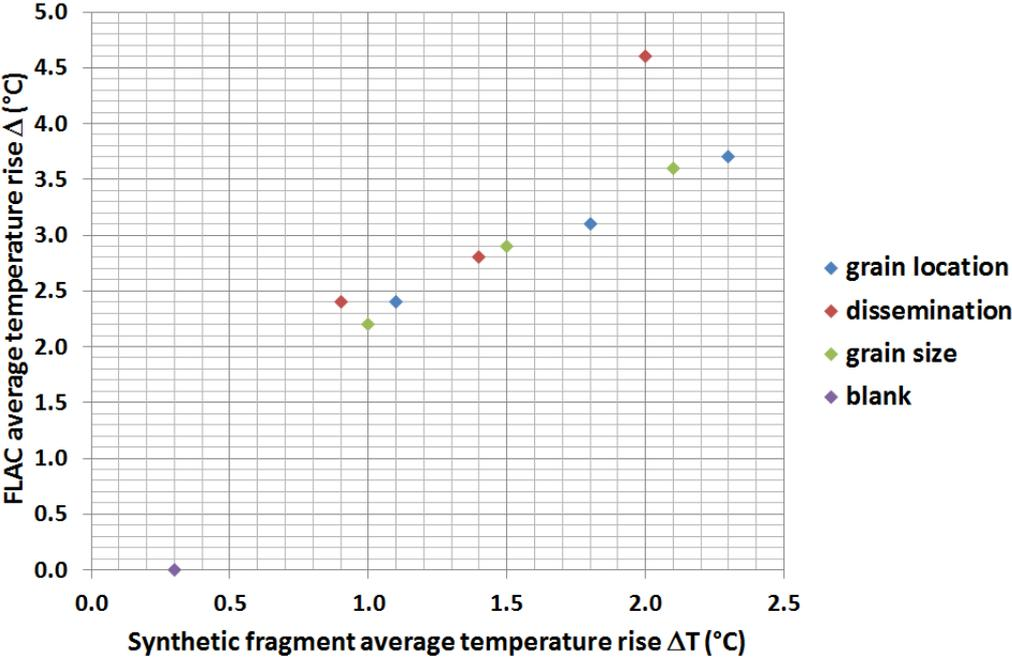
**Figure 12** Comparison of FLAC and synthetic fragment average temperature rise, 60s delay time
