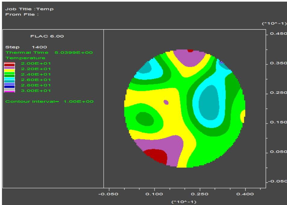
**Figure 8** Thermal profile evolution, 1% 50  $\mu\text{m}$  chalcopyrite, 100% dissemination, 5s delay time, temperature  $^{\circ}\text{C}$
