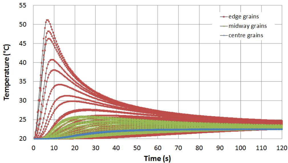
**Figure 4** Surface Heating and Cooling Profile for 1% 50 µm chalcopyrite with varying mineralisation grain location
