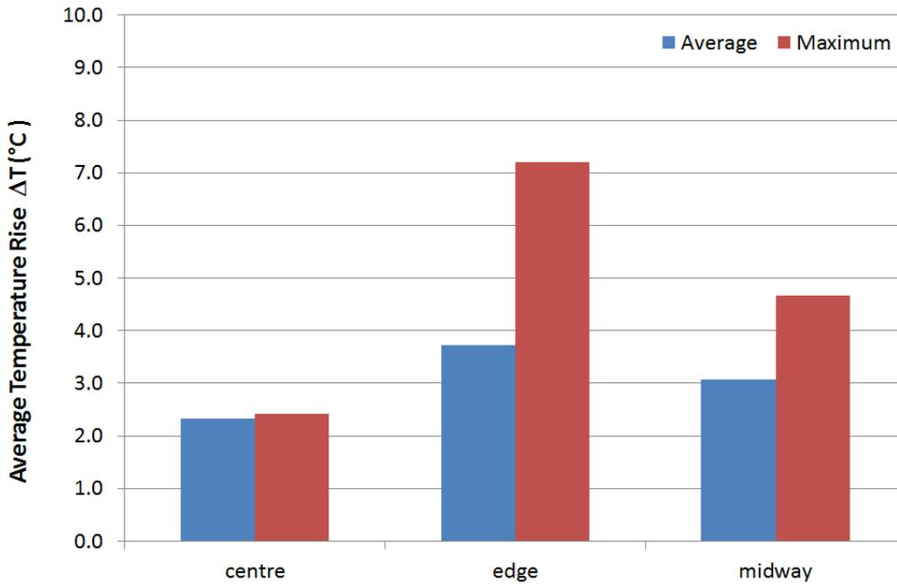
**Figure 3:** Average and maximum temperature rise around modelled fragment circumference, 1% 50  $\mu\text{m}$  chalcopyrite, varied location, 60 second delay time
