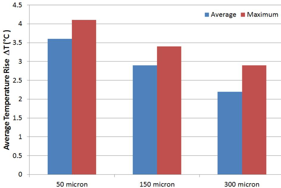
**Figure 11** Average and maximum temperature rise around modelled fragment circumference, 1% chalcopyrite, 50/150/300  $\mu\text{m}$ , 100% dissemination, 60 second delay time
