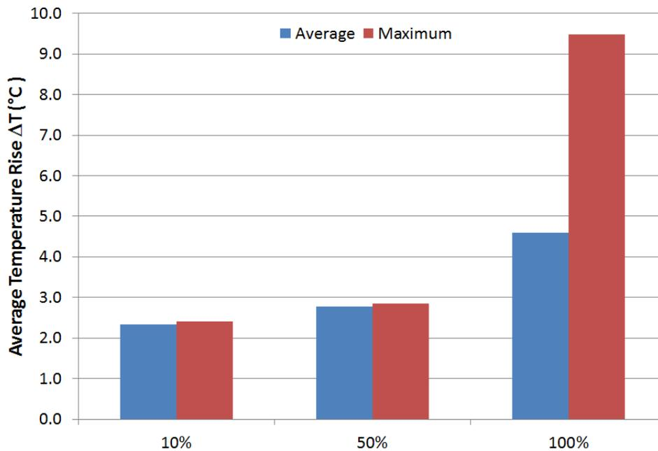
**Figure 5** Average and maximum temperature rise around modelled fragment circumference, 1% 50 μm chalcopyrite, variable dissemination, 60 second delay time
