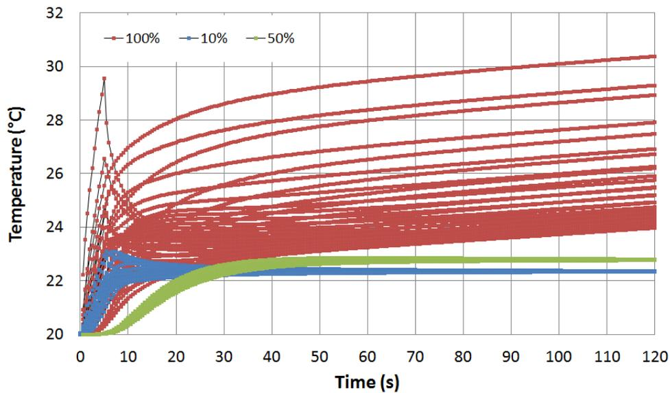
**Figure 6** Surface Heating and Cooling Profile for 1% 50 µm chalcopyrite with varying dissemination levels
