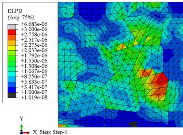
Fig. 20 local plastic dissipation energy (*ELPD* in ABAQUS).
