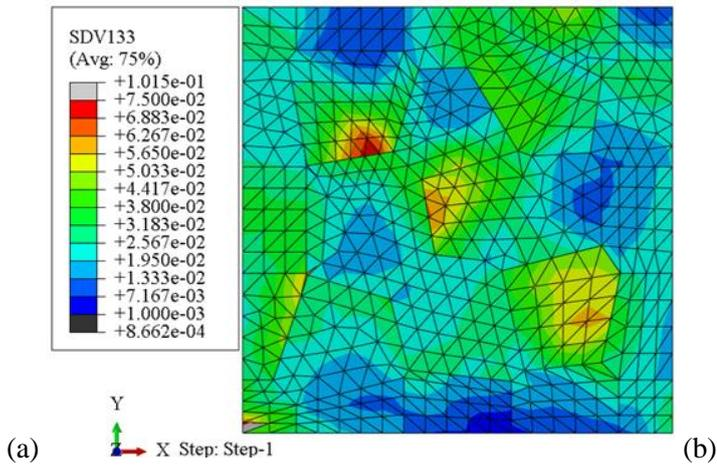
Fig. 19 The distributions of microcrack initiation indicators: (a) accumulated plastic deformation (*SDVI33* in the UMAT subroutine) ;
