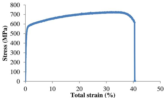
Fig. 1 Stress-strain curve in the tensile tests
