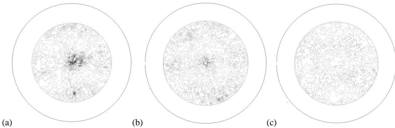
Fig. 9 Pole figures of poles: (a) {111}; (b) {200}; (c){220}.
