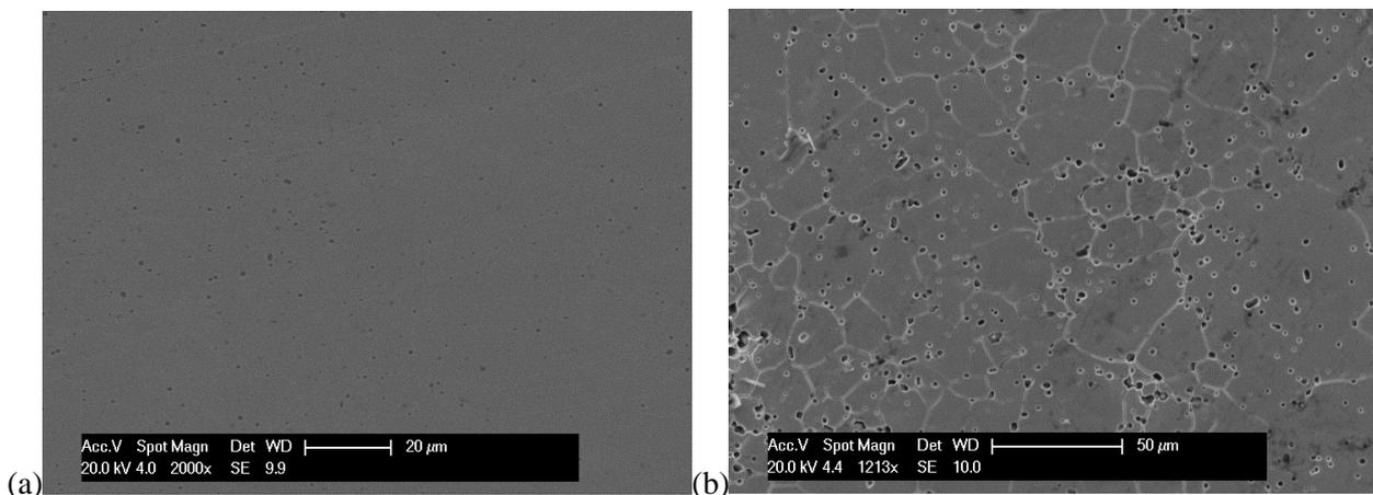
Fig. 5 SEM images for the as-received sample under the secondary electron detector (a) without etching; (b) after etching
