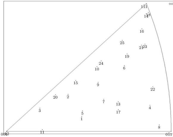
Fig. 12 The inverse pole Fig. of the loading direction, which is the y-axis of the global coordinate, generated by a MATLAB toolbox code called MTEX developed by Hielscher et al. [53].
