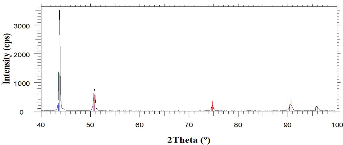
Fig. 7 Diffraction spectrum by plotting scattering angle  $2\theta$  against the relative intensity, showing red austenitic peaks and blue iron peaks from powder database spectrum.
