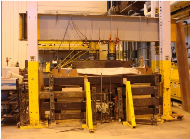
Fig. 3. Loading system installation for uniform load.
