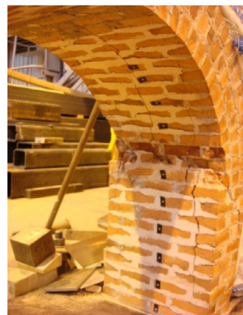
Fig. 5. (a) Deformation tendency of the tunnel; (b) crushing phenomenon at the arch springing.
