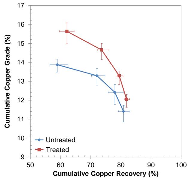
Figure 15: Coarse grind grade-recovery curves
