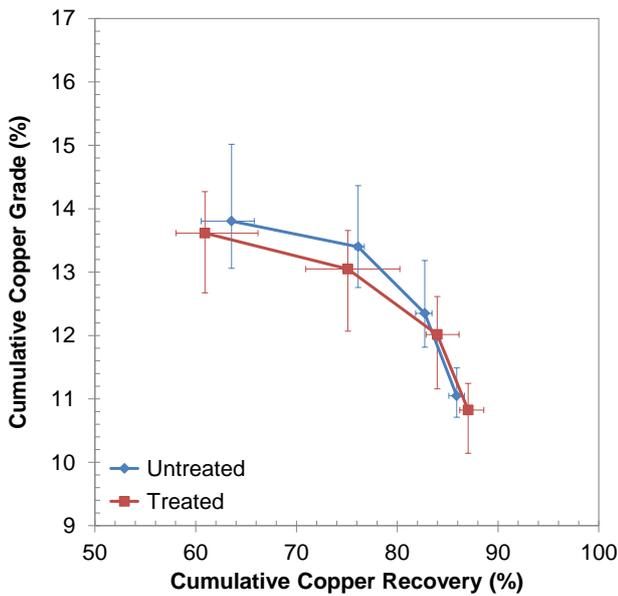
Figure 14: Fine grind grade-recovery curves
