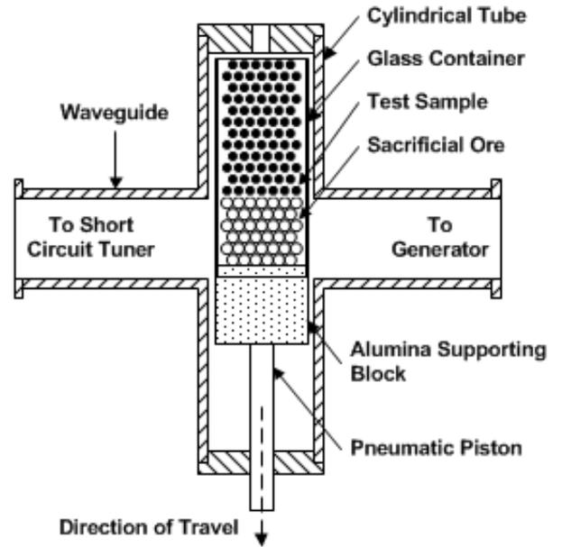
Figure 4: Single mode cavity apparatus
