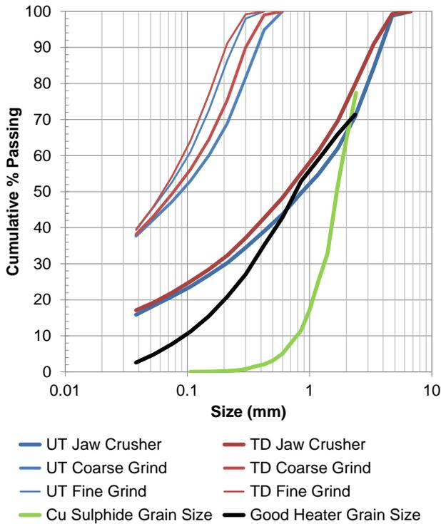
Figure 5: Crushing, grinding and native grain size distributions
