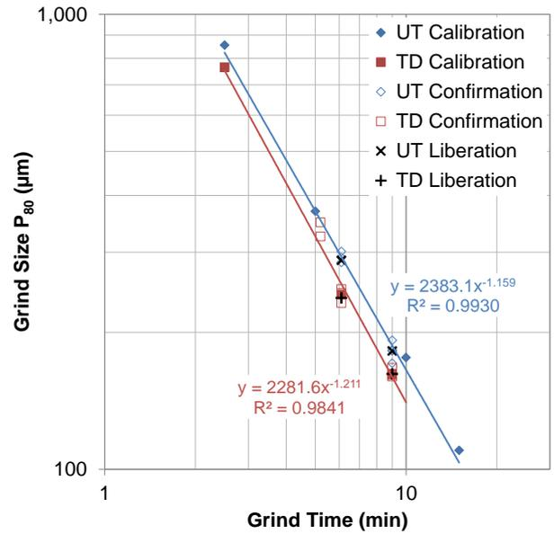
Figure 6: Grinding calibration curves
