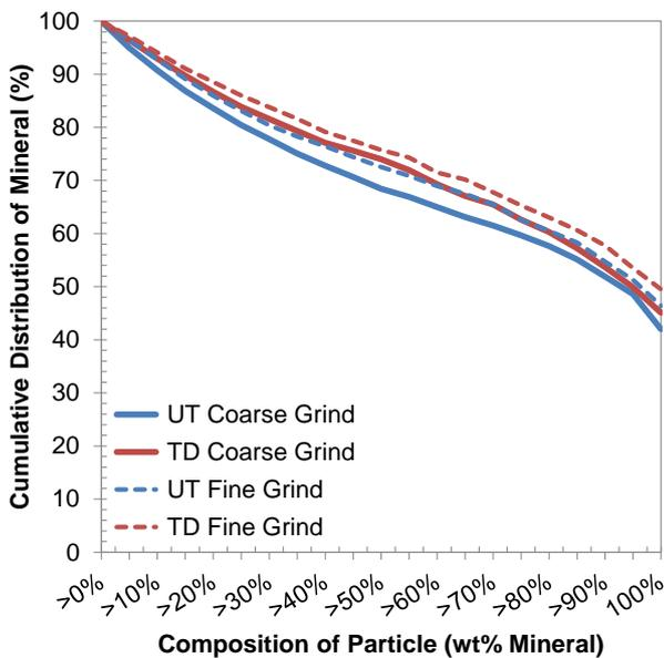
**Figure 7:** Cumulative copper sulphide liberation by composition profiles
