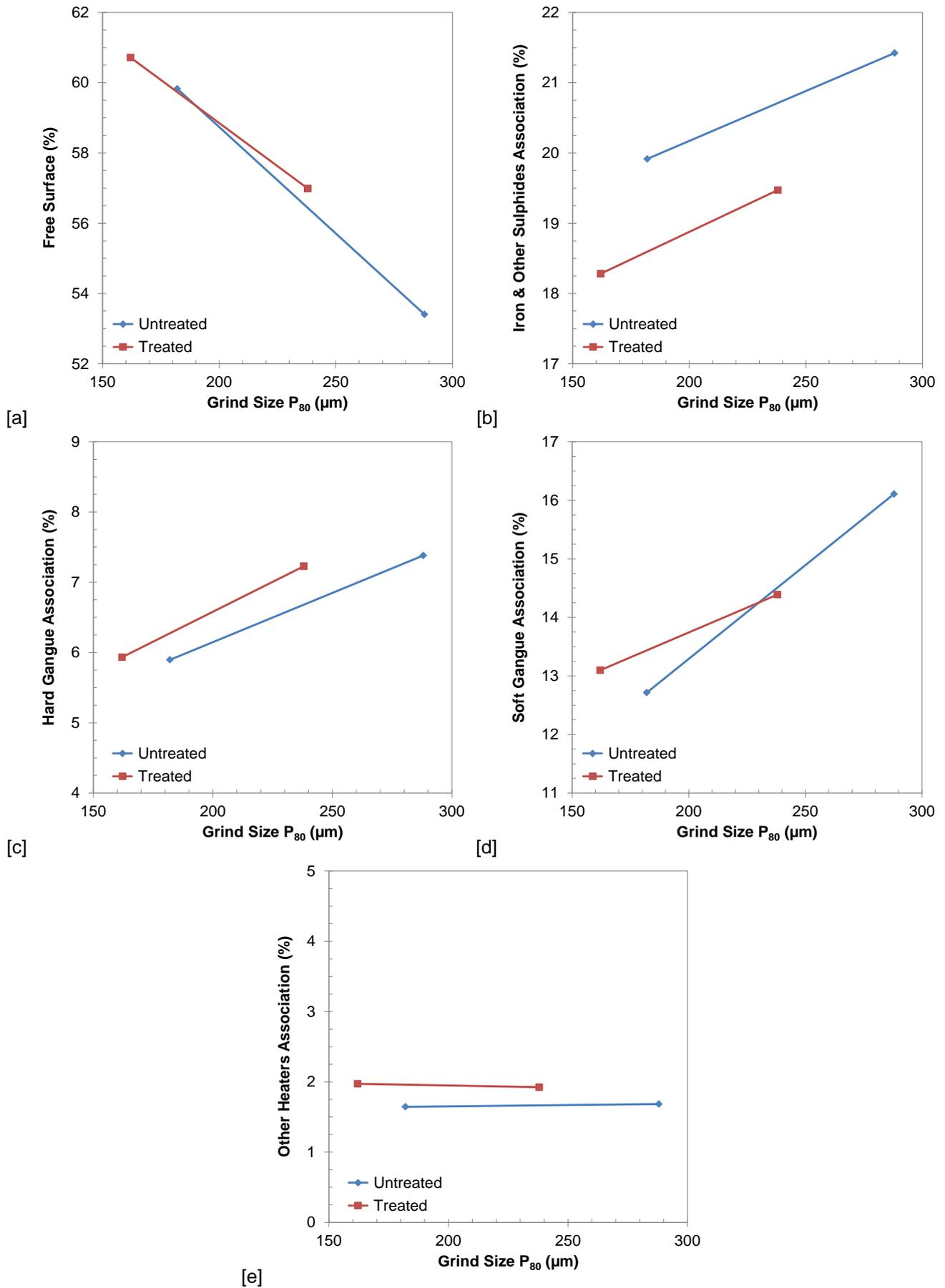
Figure 12: Change in copper sulphide associations with grind size
