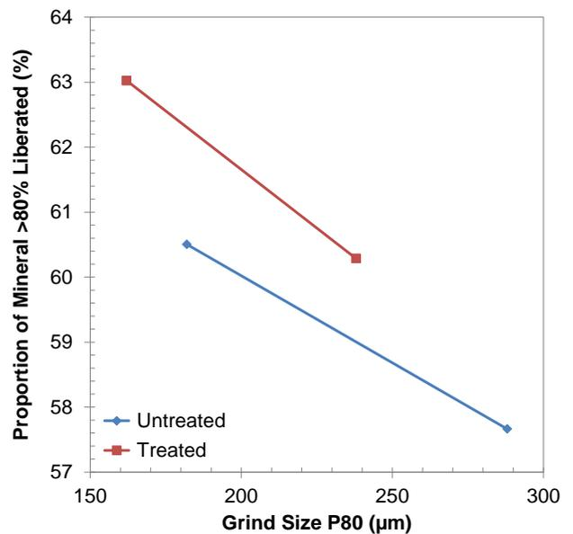
**Figure 8:** Copper sulphide liberation versus grind size
