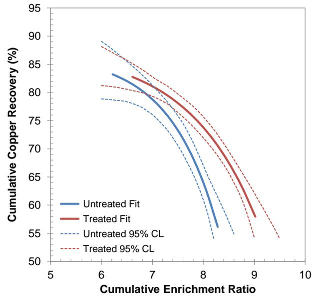
Figure 21: Fitted coarse grind enrichment ratio-recovery curves with 95% confidence limits
