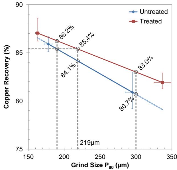
Figure 22: Copper recovery versus grind size
