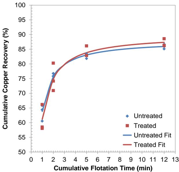
Figure 16: Fine grind copper recovery kinetics curves
