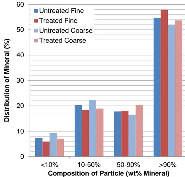
Figure 11: Absolute distribution of copper sulphide by liberation class
