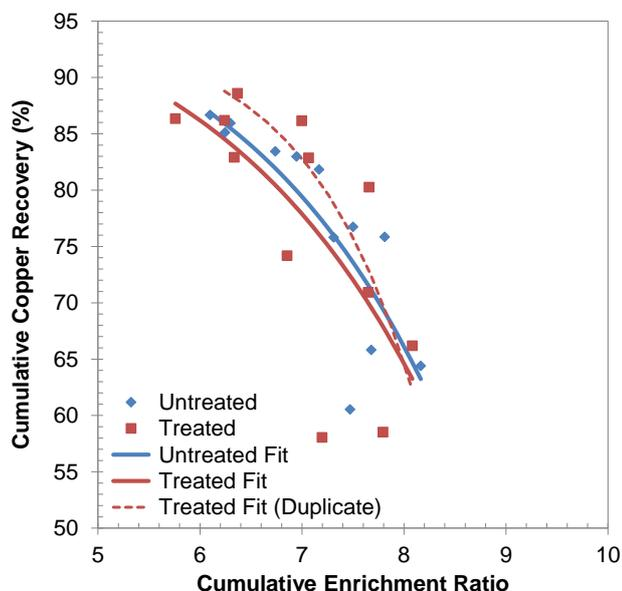
Figure 18: Fine grind enrichment ratio-recovery curves with fitted Bruey model
