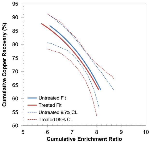
Figure 20: Fitted fine grind enrichment ratio-recovery curves with 95% confidence limits
