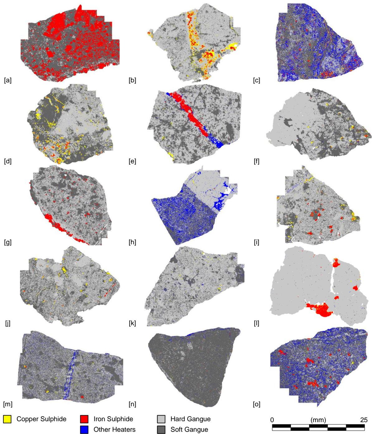
Figure 2: Example lump fragment false colour image from MLA mineralogical texture analysis
