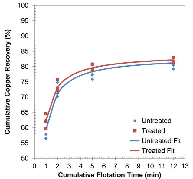
Figure 17: Coarse grind copper recovery kinetics curves
