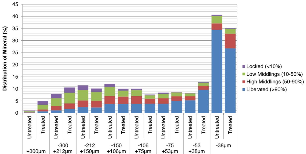
Figure 10: Absolute distribution of copper sulphide by size fraction and liberation class for the untreated fine grind vs the microwave-treated coarse grind
