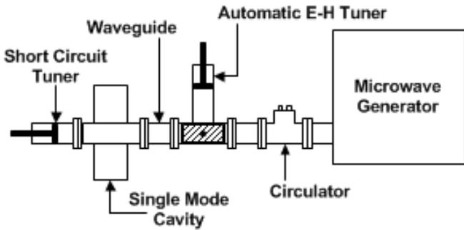
Figure 3: Microwave treatment apparatus
