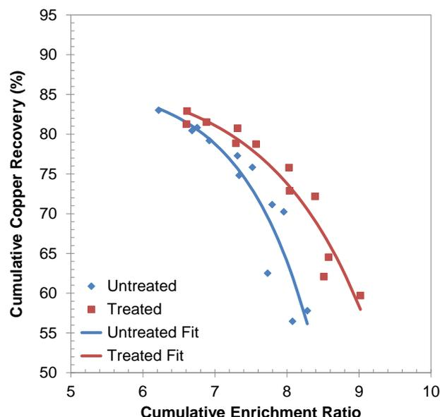
Figure 19: Coarse grind enrichment ratio-recovery curves with fitted Bruey model
