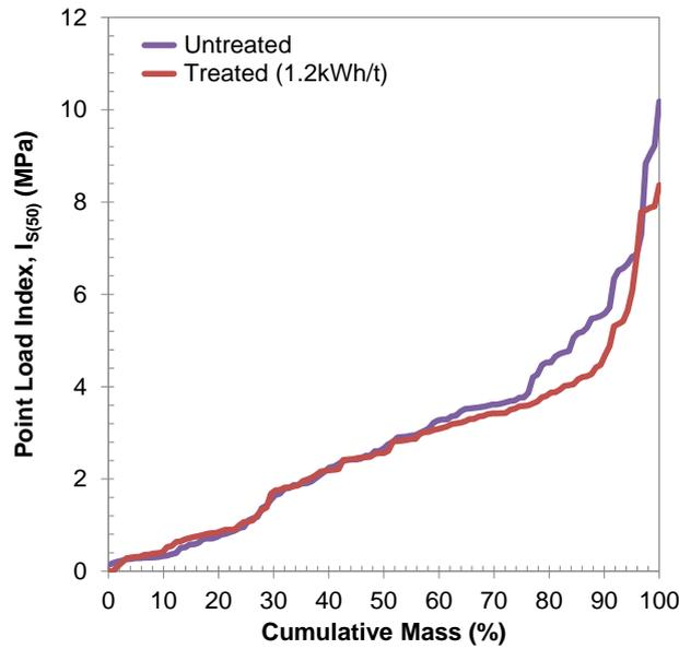
Figure 1: Point Load Test results for Cu-Ore 1
