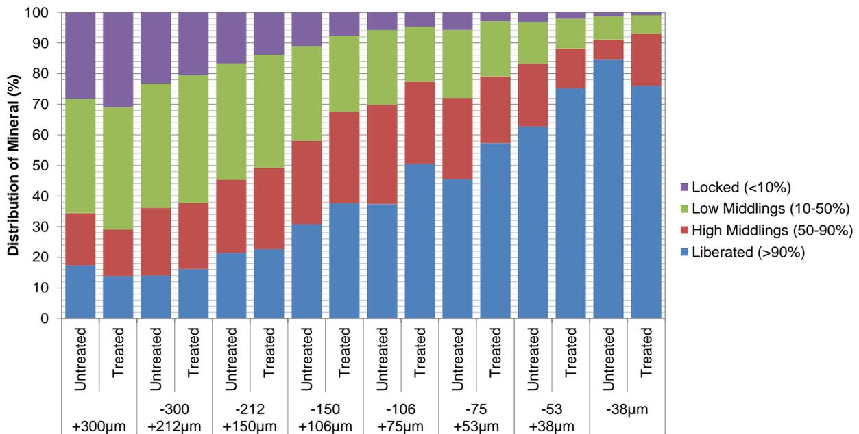
Figure 9: Distribution of copper sulphide by liberation class scaled by size fraction for the untreated fine grind vs the microwave-treated coarse grind
