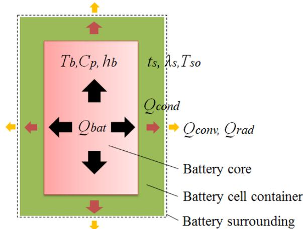
Figure 14: Heat transfer from internal battery cell to the cell container surface and to the surroundings.
