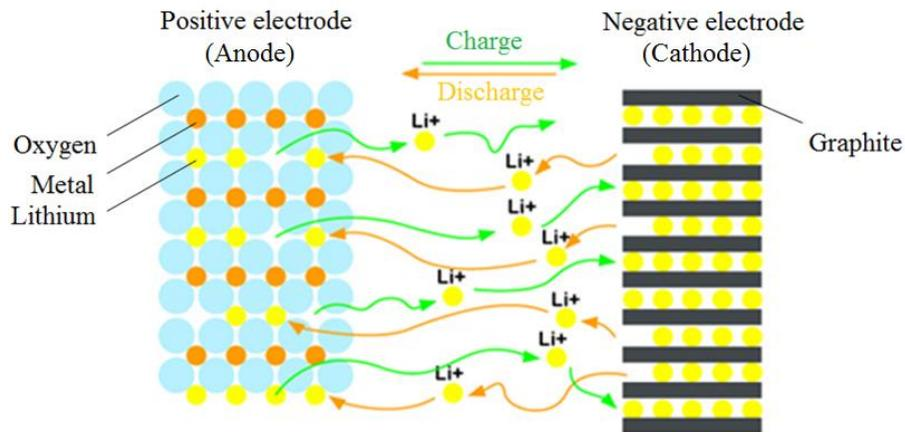
Figure 2: Lithium-ion battery mechanism during charge and discharge.
