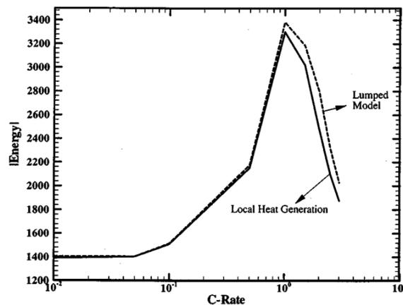
Figure 12: A comparison of thermal energy generated using local heat generation and lumped thermal models under adiabatic conditions [119].
