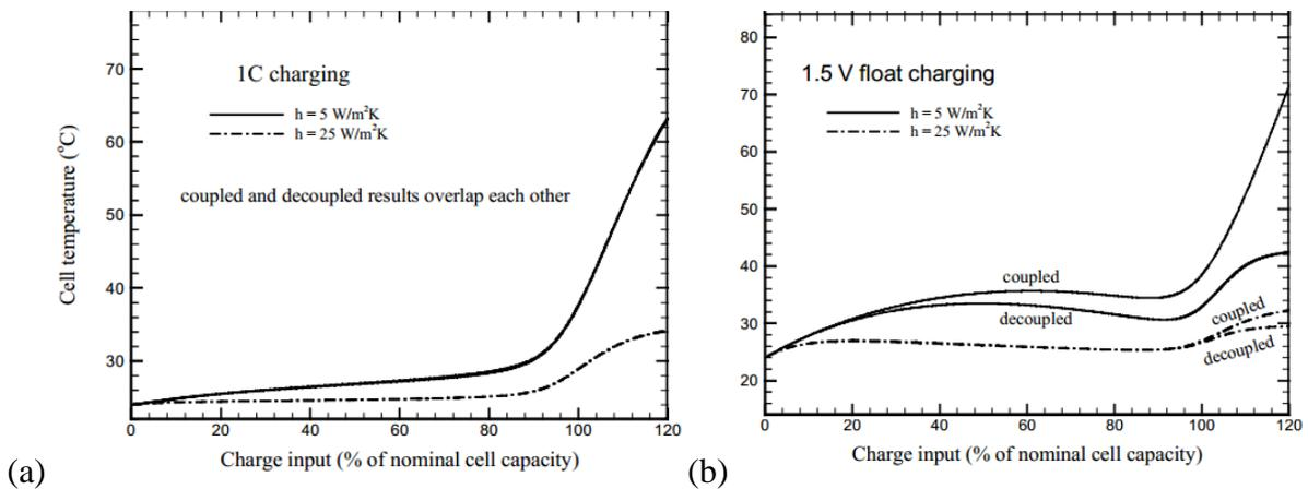
Figure 15: Comparison of predicted cell temperature between thermo-electrochemical coupled and decoupled model during (a) 1C charging and (b) 1.5V float charging [96].
