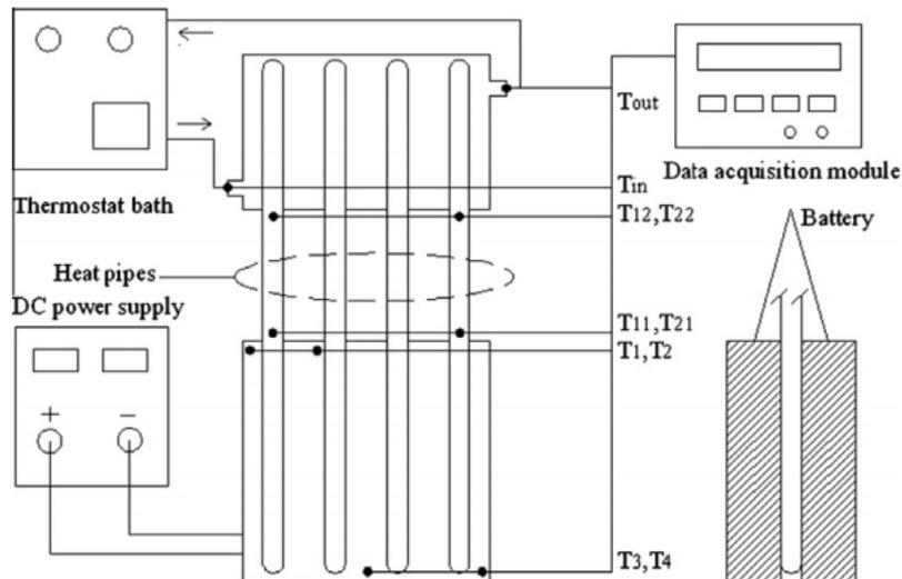
Figure 28: Cylindrical flattened heat pipe cooling for a 118\*63\*13mm 8Ah LiFePO<sub>4</sub> battery pack [210].
