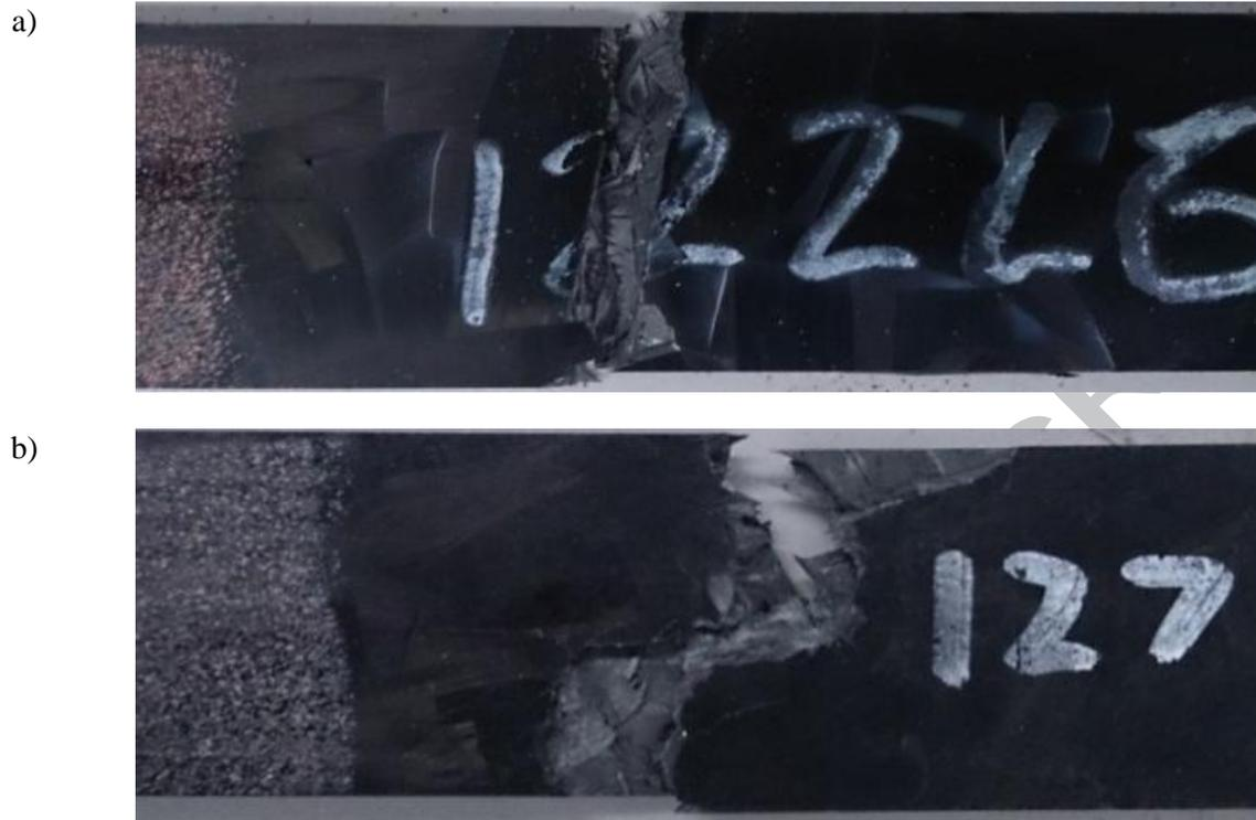
**Figure 5:** Typical failure mechanisms experienced during tensile failure of longitudinal specimens of (a) 100% mould coverage DFC, (b) 50% mould coverage DFC
