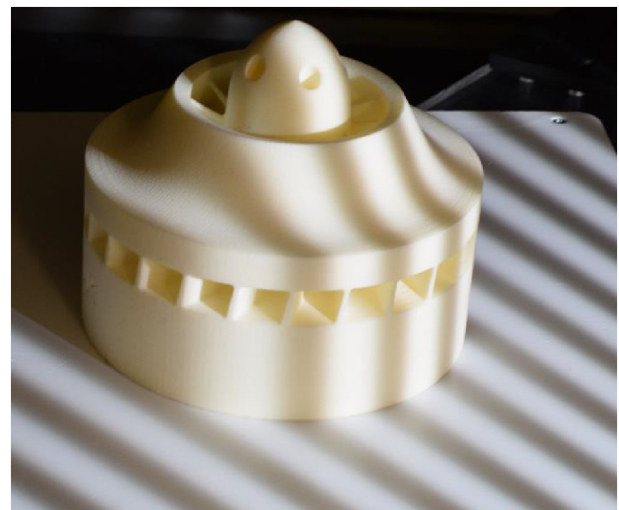
Fig. 1. A sinusoidal fringe pattern projected onto a polymer AM part from the bottom right hand corner of the image. The irradiance distribution across the part is used to reconstruct the surface.
