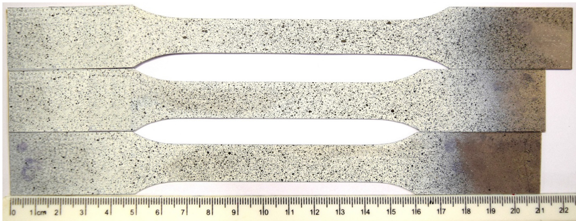
Fig. 8. Tensile specimen under different displacements to determine the VVF at nucleation.
