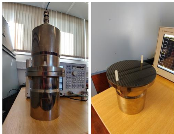
Figure 6. Coaxial unit holder manufactured according to ASTM D4935-99. On the right 3mm carbon sheet specimen in place.
