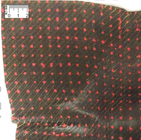
Negative shear region (top-left quadrant) (a) Reference: No risers
