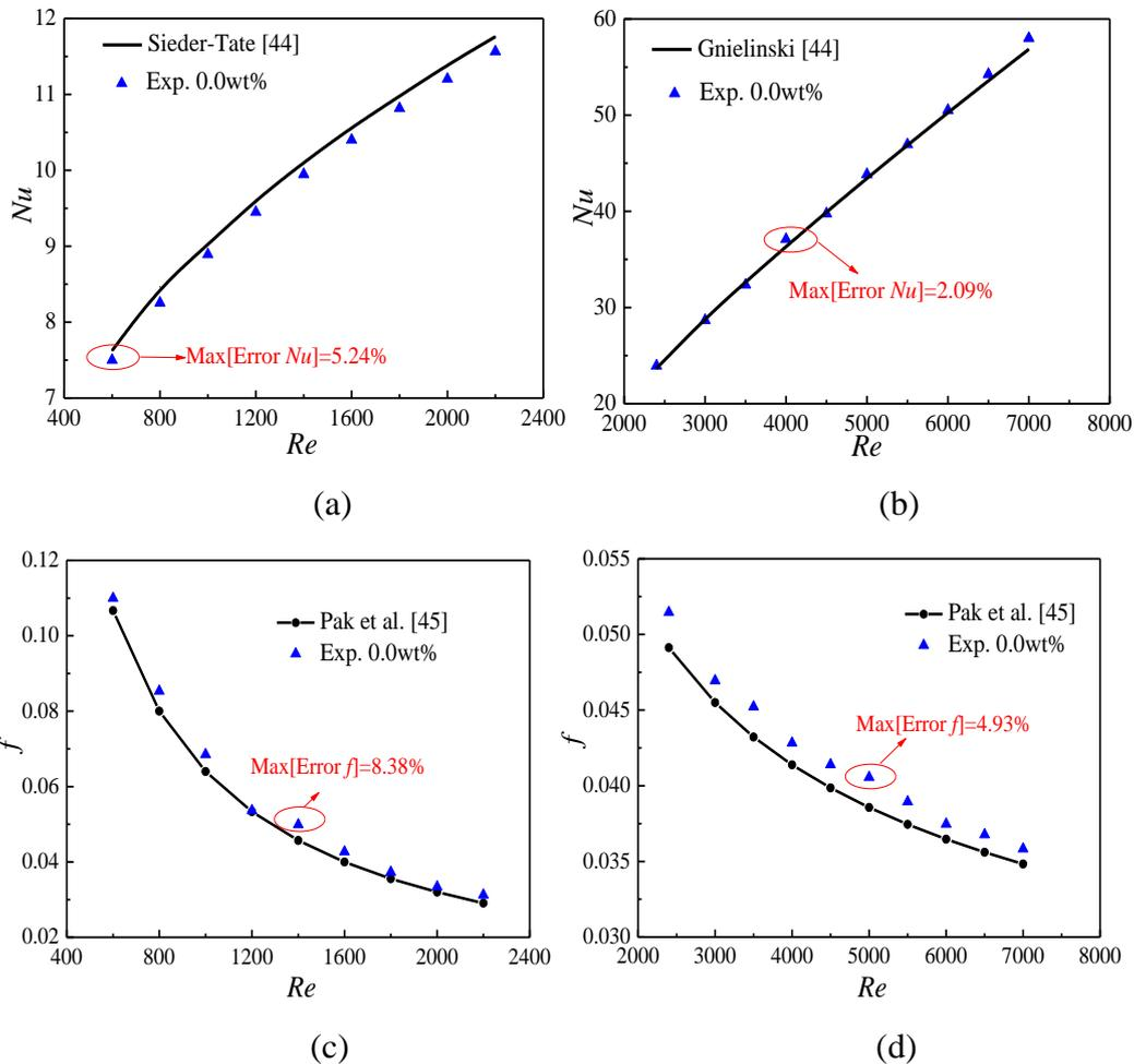
507 Figure 14 Heat transfer and flow characteristics of deionized water in a circle
