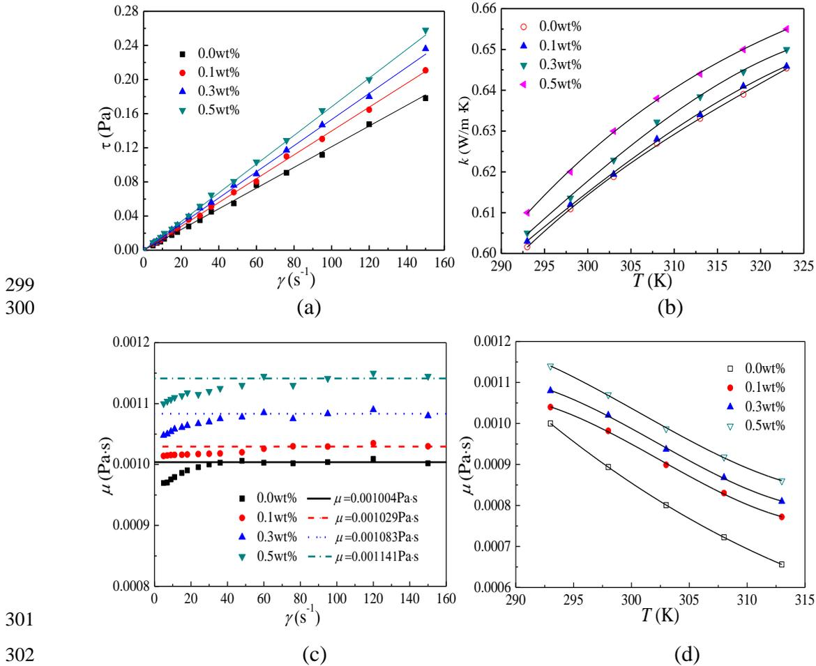
Figure 4 Thermophysical properties of  $\text{TiO}_2$ -water nanofluids (a) Newtonian-fluids characteristics at  $T_f = 293$  K; (b) thermal conductivities; (c) viscosity changes with shear rates at  $T_f = 293$  K; (d) viscosity changes with temperatures [33]
