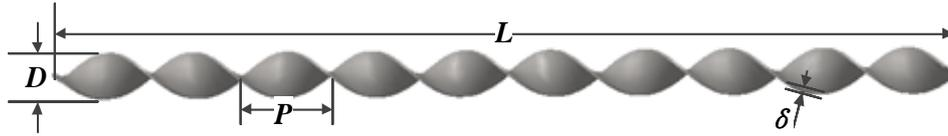
Figure 6 Structure of the twisted tape
