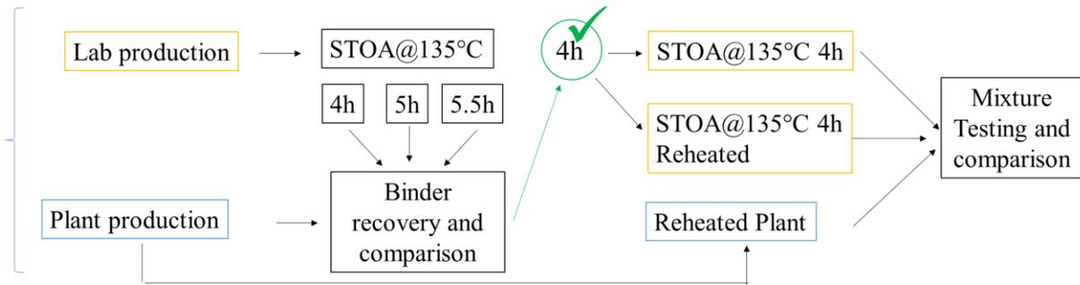
Figure 1. Short-term Aging Approach for Binders and Mixtures
