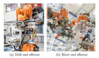
Fig. 5. Drill (on the left) and rivet (on the right) end effectors in the  ${\rm FA^3D}$
