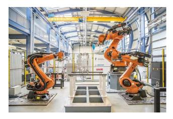
Fig. 4. Reconfigurable assembly cell of the Future Automated Aircraft Assembly Demonstrator developed by the University of Nottingham
