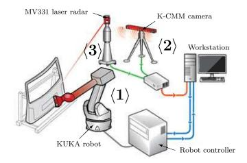
Fig. 9. Diagram of the FA<sup>3</sup>D positioning system
