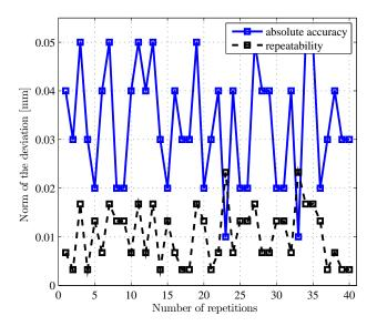
Fig. 10. Absolute accuracy and repeatability performance of the FA<sup>3</sup>D positioning system for a  $2400 \times 800$  mm aircraft component
