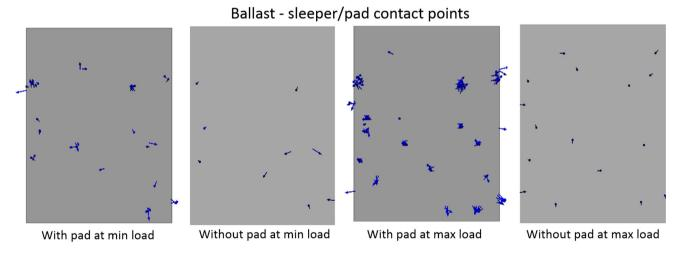
Fig. 12 The active contacts at particle-sleeper/pad interface
