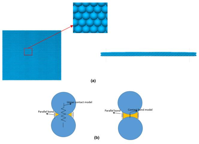
Fig. 6 a USP used in DEM simulation b The ball-ball contact model inside the USP
