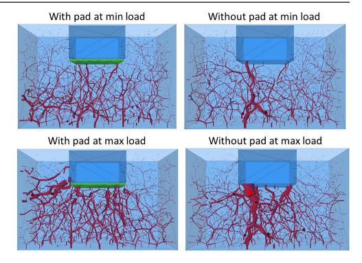
**Fig. 14** Comparison of max contact force
