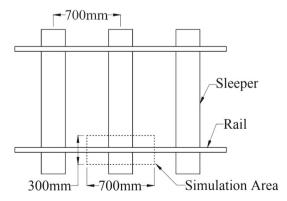
Fig. 2 Simulated track area of box test
