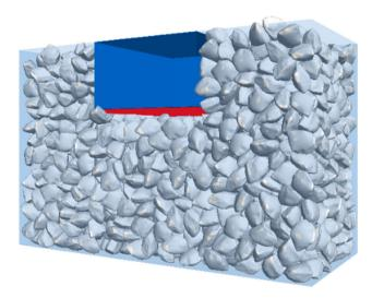
Fig. 4 DEM sample of a box test
