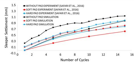
**Fig. 18** Comparison of trackbed stiffness for various pads
