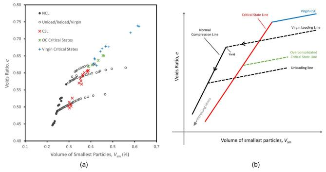
Fig. 7. Voids ratio as a function of smallest particles (a) and idealised schematic (b).
