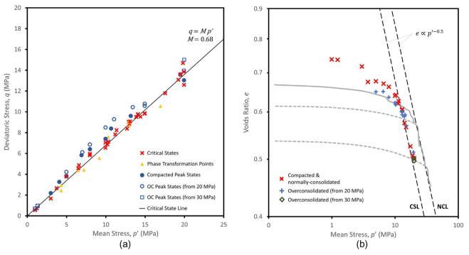
Fig. 3. Critical states from triaxial tests: q-p' axes (a) and  $\log e -\log p'$  axes (b).
