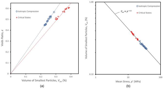
Fig. 6. Voids ratio as a function of the volume of smallest particles  $V_{sm}$  (a), and  $V_{sm}$  as a function of mean stress.
