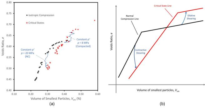
Fig. 8. Triaxial paths between states of isotropic compression and critical states (a) and schematic (b).
