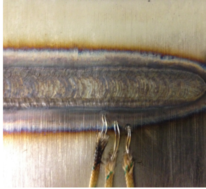
Figure 2: Thermocouples spot-welded on the top surface of the plate.
