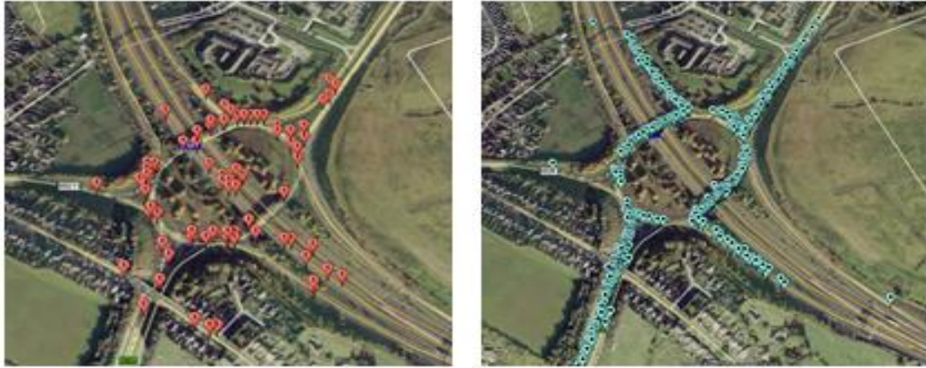
Figure 1. Grade-separated roundabout (J28 on M1 motorway, UK) with accident (left) and truck HBI (right) positions
