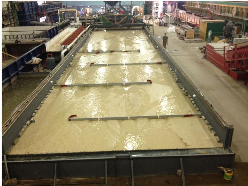
**Figure 11.** Physical model built at Colorado State University to perform ‘proof of concept’ experiments using a series of cross-valley structures to promote aggradation and build up the gradient of the sediment plain by training the braided channel of the North Fork Toutle River (NFTR) into a ‘serpentine’ course (Ettema *et al.*, 2016). [Colour figure can be viewed at [wileyonlinelibrary.com](http://wileyonlinelibrary.com)]
