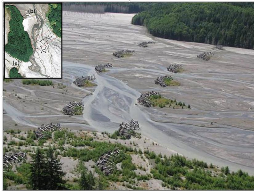
**Figure 7.** Grade building structures installed in the 2010 Pilot Project. Inset orthophoto shows (a) cutoff berm, (b) cross-valley step-weir and baffle structure, and (c) island building structures. Main picture shows Engineered Log Jam island building structures in area outlined in red in the orthophoto three years after their installation. [Colour figure can be viewed at [wileyonlinelibrary.com](http://wileyonlinelibrary.com)]
