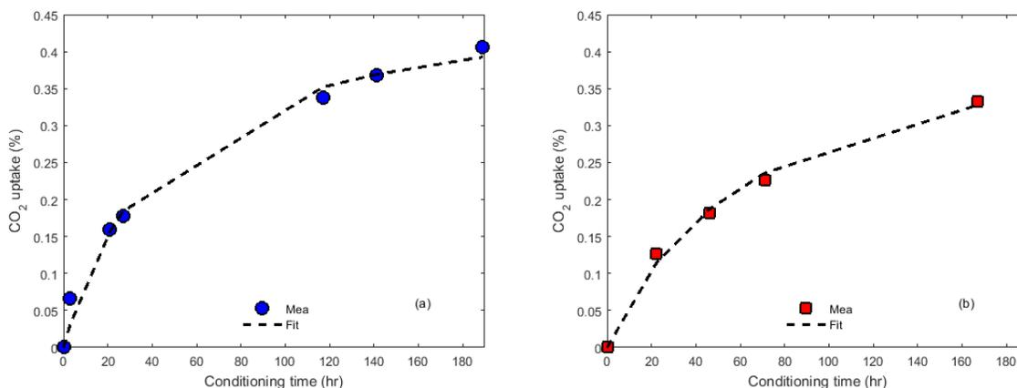
**Figure 6.** Pelleg model fit to CO<sub>2</sub> uptake by bitumen at 25°C and 40 psi. a) 190 Pen, model parameters were:  $C_1=90.6612$  and  $C_2 = 2.0666$ , b) 50 Pen, model parameters were:  $C_1=146.4474$  and  $C_2 = 2.1763$ .
