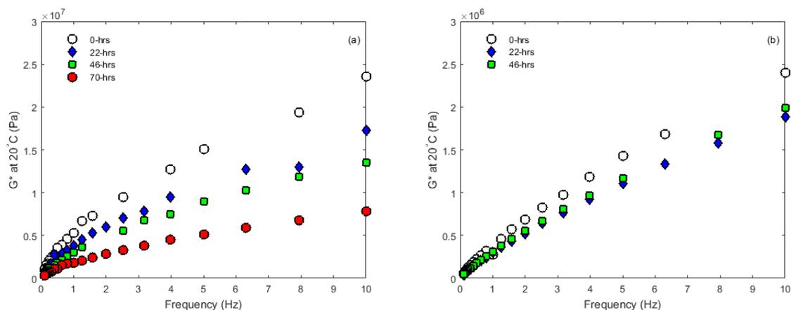
**Figure 9.** Complex shear modulus for  $\text{CO}_2$ -modified bitumen showing the viscosity-reducing (softening) effects of pressurized (40 psi)  $\text{CO}_2$  dissolved in bitumen. a) 50 Pen bitumen. b) 190 Pen bitumen.
