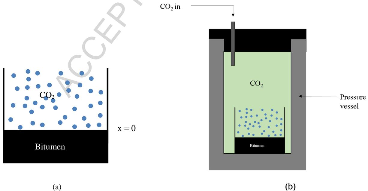
**Figure 2.** Schematic of bitumen specimen in an impermeable aluminum can that was used for CO<sub>2</sub> diffusion experiments. The tests were conducted in a pressured vessel (b) maintained at a constant pressure so that the concentration of CO<sub>2</sub> at the bitumen-CO<sub>2</sub> interface remained constant throughout the test and thus ensuring a one-dimensional diffusion.
