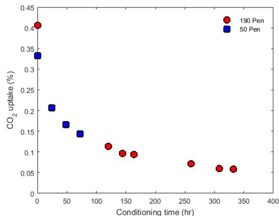
**Figure 8.** Desorption rates of CO<sub>2</sub> from modified bitumen under ambient conditions. Bitumen samples were previously conditioned in CO<sub>2</sub> at 40 psi for up to 200 hours prior to desorption experiments.
