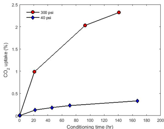
**Figure 18.** Effect of conditioning pressure on CO<sub>2</sub> uptake for 50 Pen bitumen.
