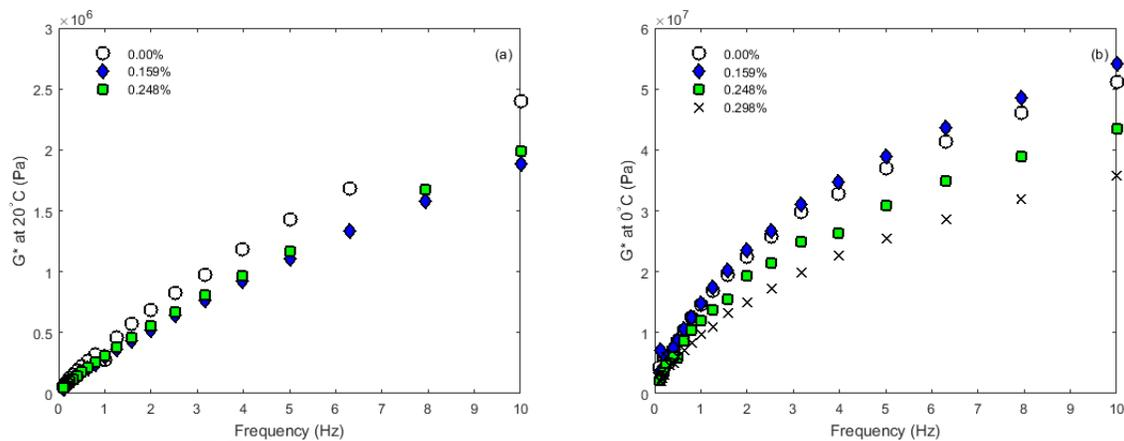
**Figure 10.** Complex shear modulus data at two tests temperatures for 190 Pen bitumen modified with CO<sub>2</sub> gas at injection pressure of 40 psi. a) 20°C; b) 0°C. Note that CO<sub>2</sub> uptakes of 0.000%, 0.159%, 0.248% and 0.298% correspond to conditioning time of 0-hours, 20-hours, 50-hours and 70-hours, respectively.
