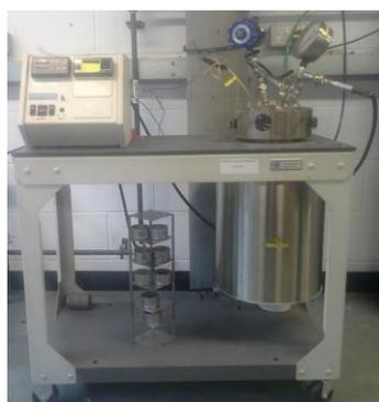
**Figure 4.** Modified SATS test set-up consisting of pressure vessel, pressure and temperature controllers, and bitumen sample holder for producing CO<sub>2</sub>-modified bitumen.
