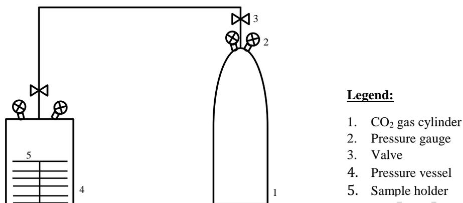
**Figure 3.** Schematic of the CO<sub>2</sub> system used for modifying bitumen.
