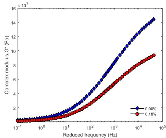
**Figure 13.** Complex shear modulus master curve for 50 pen at two CO<sub>2</sub> concentrations. Reference temperature: 20°C.
