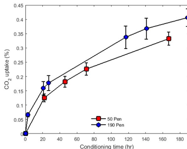
**Figure 5.** *CO<sub>2</sub> diffusion kinetics in bitumen at 20°C and 40 psi. Error bars represent one standard deviation of the mean. CO<sub>2</sub> uptake was observed to be higher in the softer 160-220 pen bitumen than in the harder 40-60 pen bitumen.*
