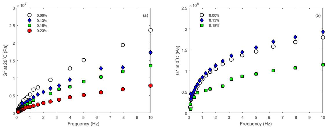
**Figure 11.** Complex shear modulus data at two tests temperatures for 50 Pen bitumen modified with  $\text{CO}_2$  gas at injection pressure of 40 psi. a)  $20^\circ\text{C}$ ; b)  $0^\circ\text{C}$ . Note that  $\text{CO}_2$  uptakes of 0.000%, 0.130%, 0.180% and 0.230% correspond to conditioning time of 0-hours, 20-hours, 50-hours and 70-hours, respectively.
