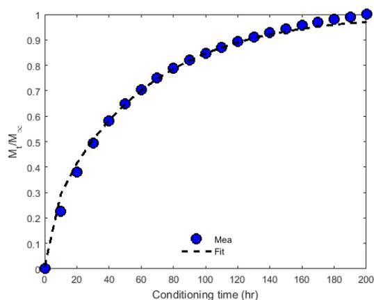
**Figure 7.** Fick's law fit to CO<sub>2</sub> uptake showing a good fit. Data for 190 pen at 25°C and 40 psi.
