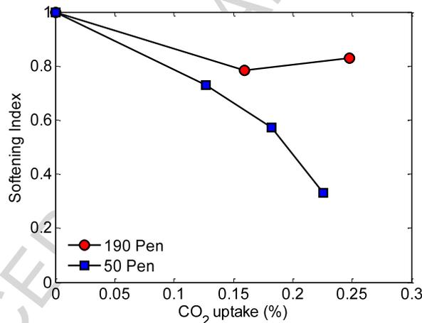
**Figure 12.** Softening indices for complex shear modulus of bituminous binders showing the viscosity-reducing effect of CO<sub>2</sub> at 40 psi and 20°C in bitumen. Complex shear modulus data were obtained at 20°C and 10 Hz.
