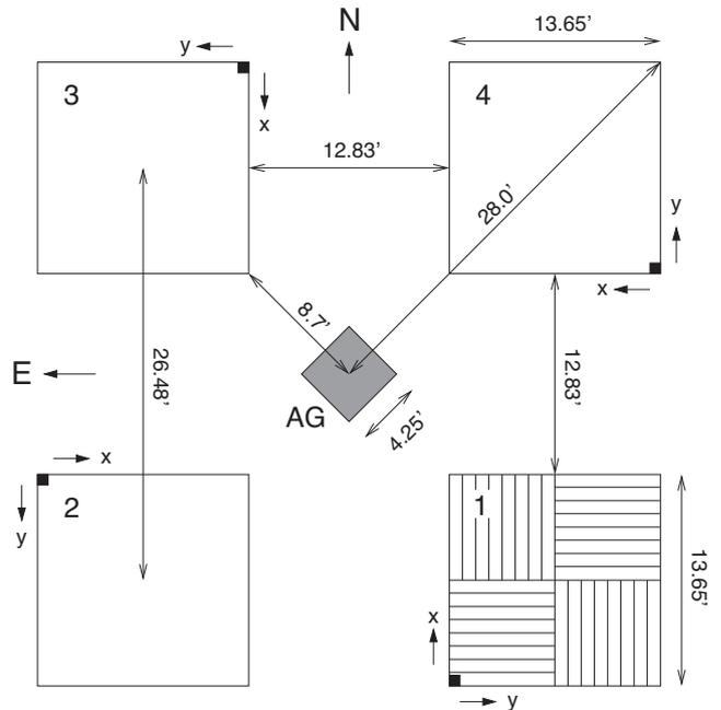
**Figure 1.** The WFCAM focal plane showing the four detectors and the autoguider (AG). Numbering of detectors is the same as that used in the WSA and for extension numbering in the multi-extension FITS image files. Detectors are divided into four quadrants, each quadrant having eight channels as illustrated in detector 1. Note the convention used for the image pixel coordinate system in each detector. In this figure taken from Dye et al. (2006), north is upwards and east is to the left.
