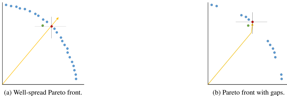
Figure 22: Example of an inaccurate objective-function on a Pareto front that is well-spread (a) and on a Pareto front with gaps (b).
