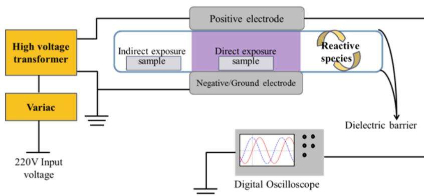
Figure 2. Schematic of the dielectric barrier discharge (DBD)-setup for the generation of plasma treated water (PTW-DBD).[18]
