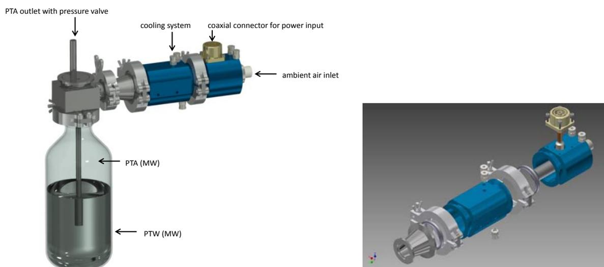
*Figure 1.* Left: Schematic of the microwave-setup for the generation of plasma treated water (PTW-MW).<sup>[16]</sup> Right: exploded drawing of the plasma source PLe<sub>xc</sub><sup>[29]</sup>
