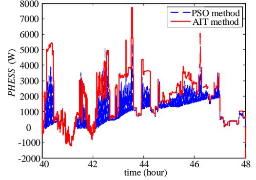
Fig. 8. Power output of HESS with PSO and with AIT
