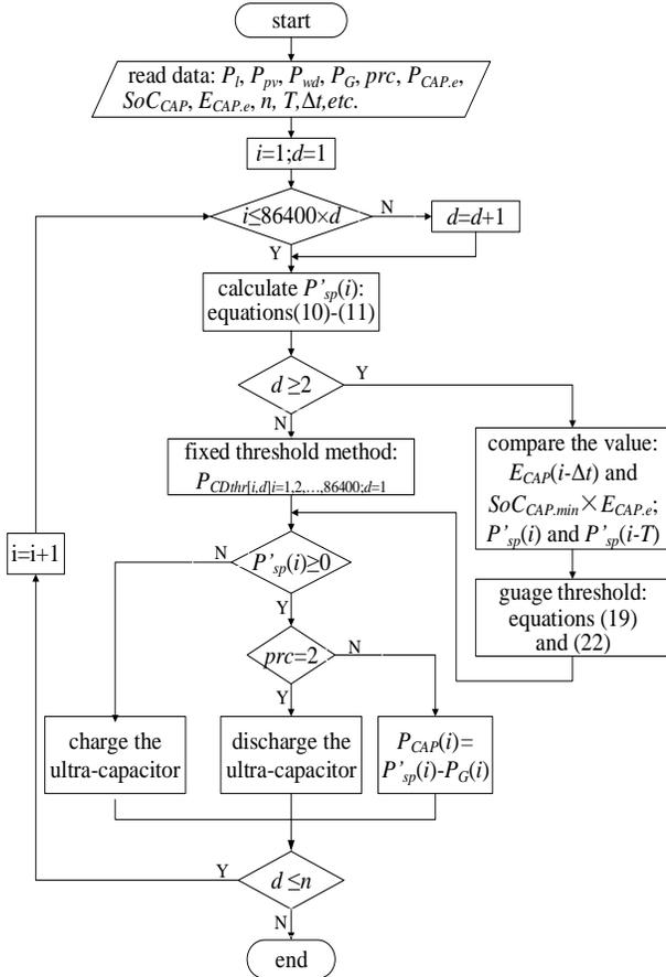
Fig. 2. Algorithm for ultra-capacitor Management System
