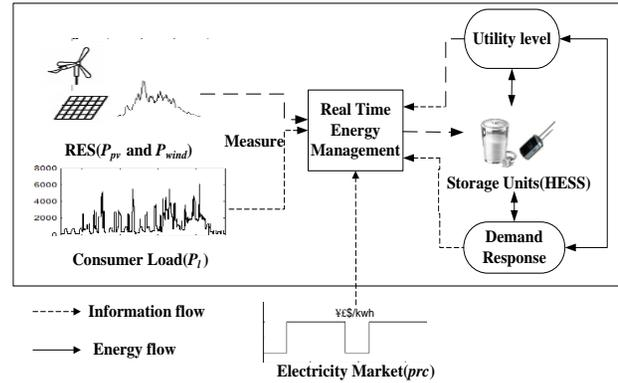
Fig. 1. Structure of Energy Management System
