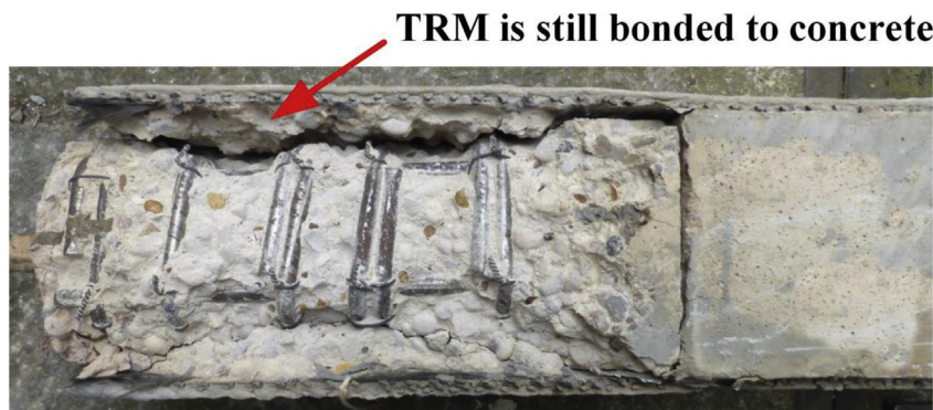
Fig. 17. Exploded specimen heated up to 550 °C.
