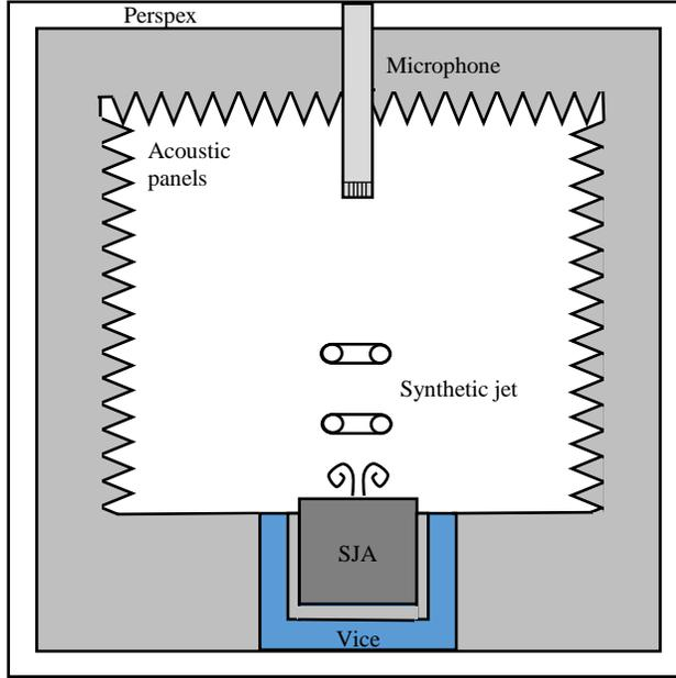
**Figure 8. Test rig for SJA noise measurements**
