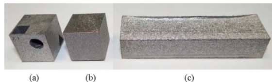
Figure 1. Pictures of the samples: (a) Al-Si-10-Mg, (b) Ti-6Al-4V LPBF cubes and (c) Ti-6Al-4V EBPBF rectangular prism.
