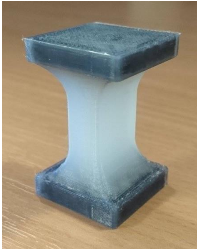
Figure 8: Set 1 (0% carbon fibre) specimen with reinforced bases.
