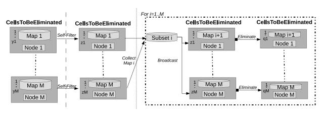
Fig. 3. Stage 3: An iterative Spark approach to remove redundancies from the same dataset: CellsToBeEliminated. Note that in the plot y > z > q.
