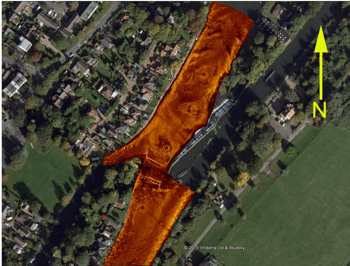
Figure 16 – Four 50 metre radius scans mosaicked to provide a plan of the submerged structure of the historic Sunbury Weir in the River Thames built in 1812. The edges and floor of the river channel are clearly defined and evidence of the remnants of dredging can be seen in the upper northern part of the scan.
