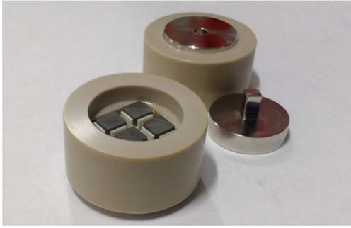
Fig. 2. Picture of the evaluated multiple and single chip SiC Schottky diode modules using pressure contacts in different assembly stages
