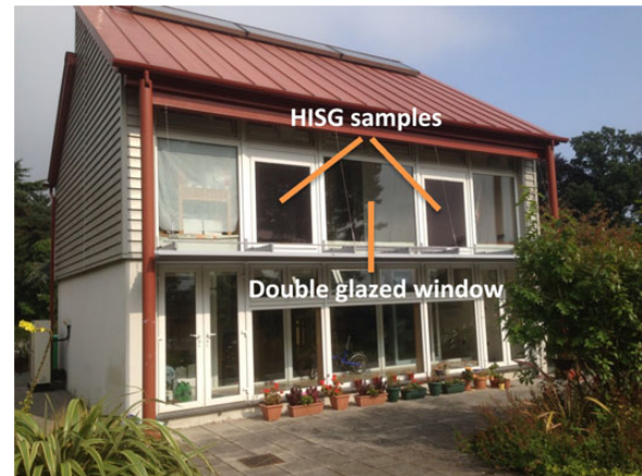
Figure 3. In situ testing of HISG through creative energy homes at the University of Nottingham.
