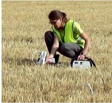
FIGURE 1 A Bruker Tracer IV-SD hand-held XRF spectrometer, deployed at Nuthampstead airfield (August 2015). Here, the Bruker spectrometer is held in the operator's right hand, and the 3 V Vacuum Pump in their left [Colour figure can be viewed at wileyonlinelibrary.com ]
