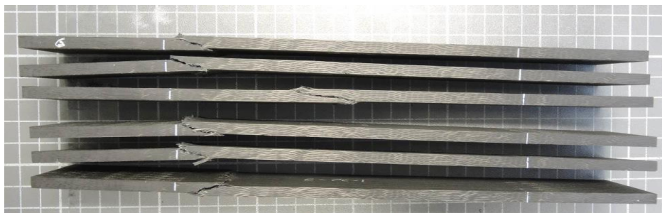
Figure 8: An example of the coupon tests (in plane compression).
