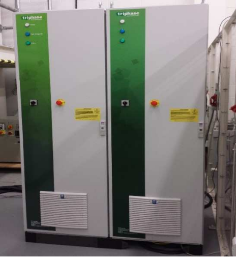
Fig. 10. Controllable Power and Voltage Source (Triphase).
