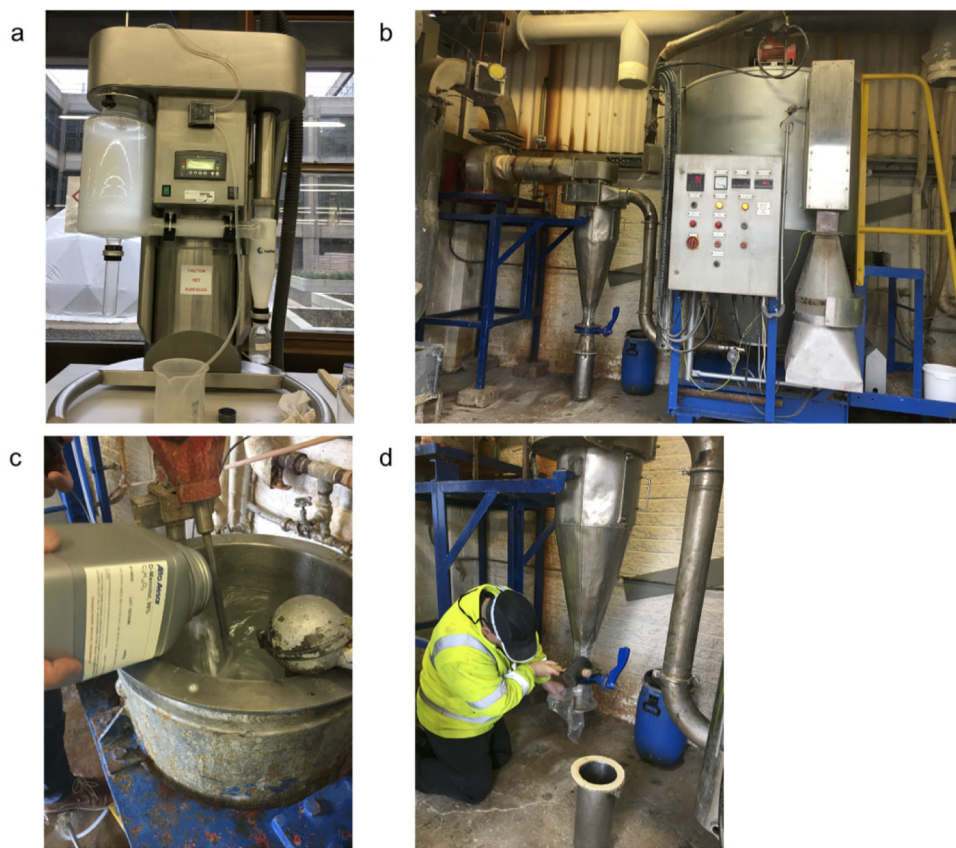
FIG 1 Images of the equipment used for spray drying phages. (a) Laboratory scale spray dryer used to dry phages SPFM10 and SPFM14. (b) Industrial spray dryer used to dry the phages that were then added to the weaner meal and pelleted. To dry the phages in the industrial scale dryer, the excipients, phages and water were mixed together in vessel (c) and dried powder was collected in tube (d).
